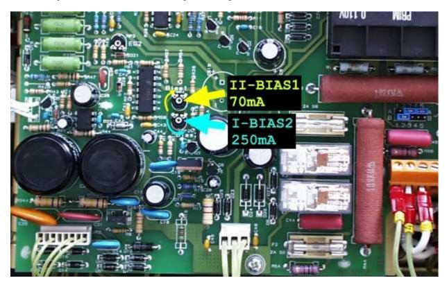
Please note that RP2 will affect both levels, while RP1 - only the low level of the idling current. That is why, the high level is adjusted the first, and only then is set the low level (according to the procedure described below).
