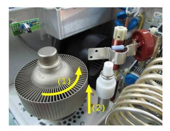
While holding the tube for the heat sink, turn it to 120° (a third of a full turn) and counter clockwise, in order to release the tube from the socket spring contacts. Be sure to avoid overstraining the contacts while pulling the tube vertically up until you get it out of the socket.
