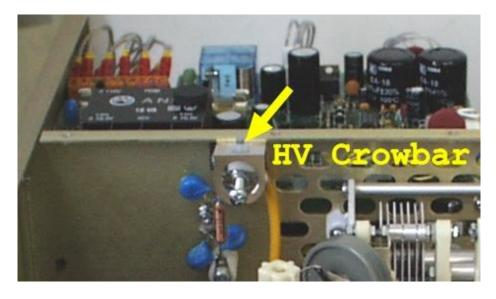
Check whether the HV LID crowbar makes a reliable short-circuit across the HV wiring when the cover is missing.
