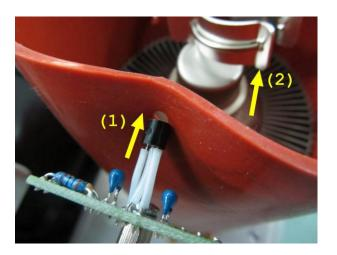
Unclip the anode spring clip from the tube cap - look at the yellow arrow (2) above - and then unthread the rubber chimney out of the anode heat sink (together with the anode spring clip inside). Keep an eye on the temperature sensor.
