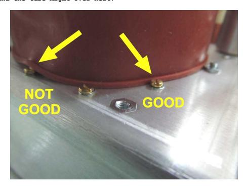
At last, install the UHF suppressor stripe using two original screws and lock washers (should have been preserved at previous steps). Tighten the screws properly.
