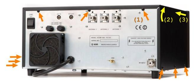
Lift the rear edge of the cover slightly (to 2-3cm) and then pull the cover backwards, in order to release it from front-panel's chutes. Remove the top cover.
