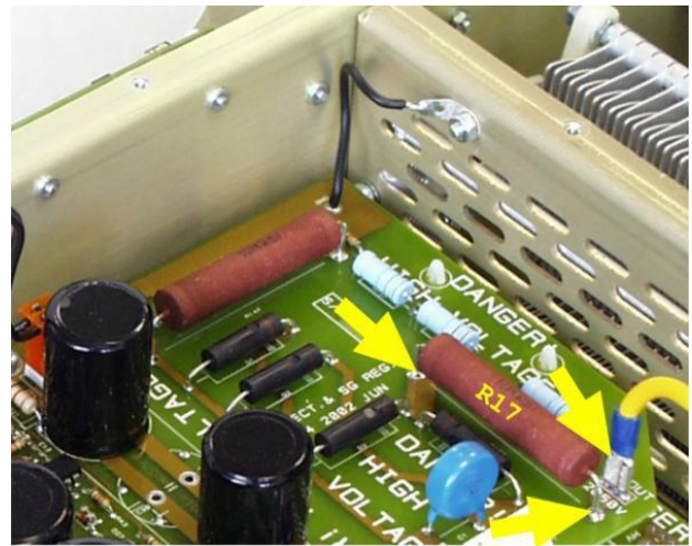
Fig.2 High Voltage Points to discharge on HV Filter or HV&SG PCBs
