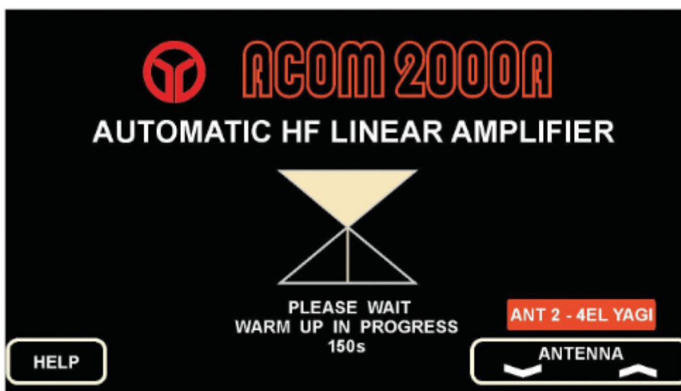
Figure 4-1 RCU display during warm-up
