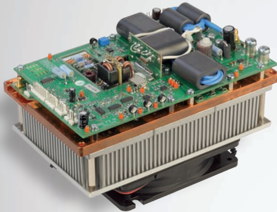
High Power Amplifier Units
