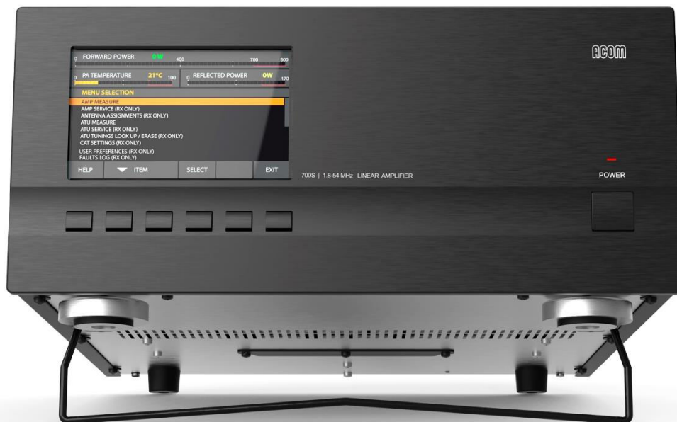
Figure 2-3 | Front panel - Ergonomic position with tilt foot bar
