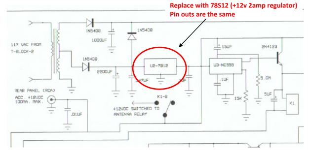
At that point I decided that the problem was the regulator was not sufficient to drive the four new bulbs. No info existed on the old original bulbs so I presume they were fairly low wattage, maybe even 1 or 1.5w. I then took out the control board. This is also not easy as all connections are hard wired. I had to un-solder some connections from the main board to allow for full removal.
