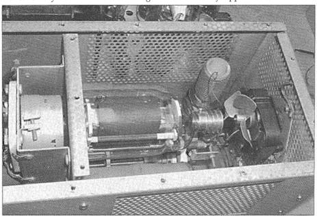
A shiny 813 is reinstalled in the PA cage, and waits for its voltages to be applied.
