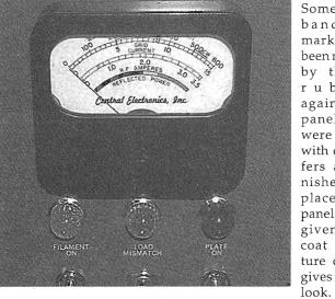
The large multimeter and knobs were cleaned and polished using a light polishing compound and set aside for later assembly. They now looked like new.
