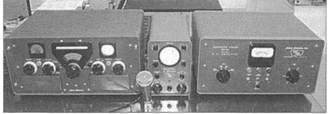
This is how my restored Central Electronics station looks. Left to right, 200V transmitter, MM1 station monitor, and the 600L linear. An Electro-Voice 667 microphone completes the station. View below is underneath the chassis.
