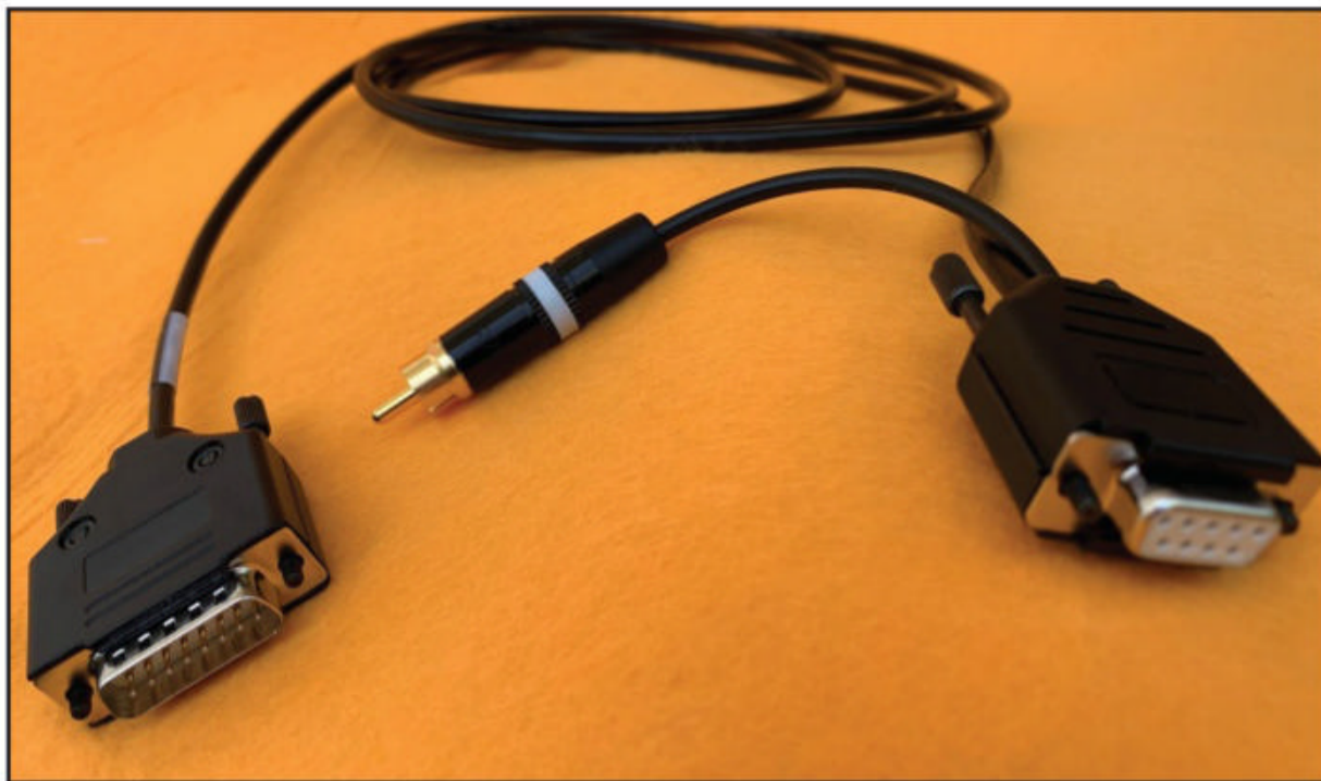
Photo C. The 08-07662-001 HPA cable provides the communication between the HPAC and the Ameritron amplifier.
