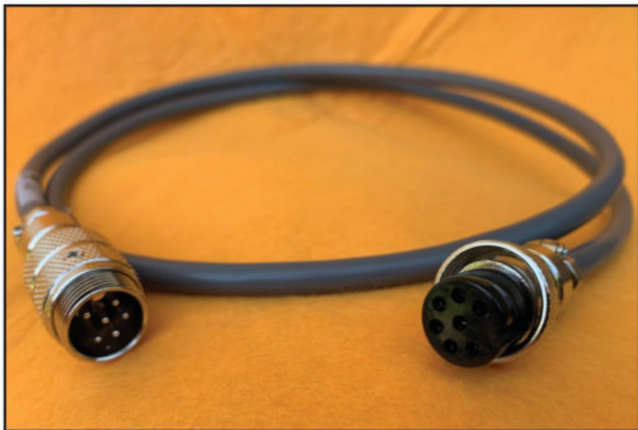
Photo B. The 08-05956-001 cable connects the transceiver to the HPAC.
