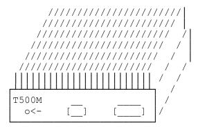
2-30MHz, 4x 150W push pull amps in parallel. > 10dB gain, 70W max drive. (typical 15-40W) IMD 3rd Order >-32dB @-500W, >-36dB @ 400W. PA harmonics to better than -43dB. 13.6V @ 75 Amps needed for full 600W output! 1kW DC input, Infinite SWR rated, <2:1 recom. 15A charger & car battery will power it (SSB). Thermal 70°C heatsink shutdown. CW/SSB use! Over current 75A trip (high SWR & over drive). Manual & Remote operation (On & Band select). Weight 8kg.
