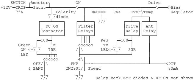
Added components mounted on or near the band switch.
