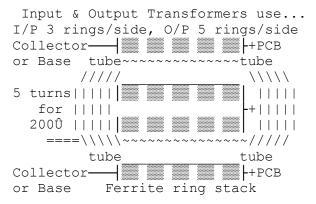
The inputs & outputs are wired up from the drive splitter & output combiner with staggered wire lead lengths, so all the RF signals ends up exactly in phase.
