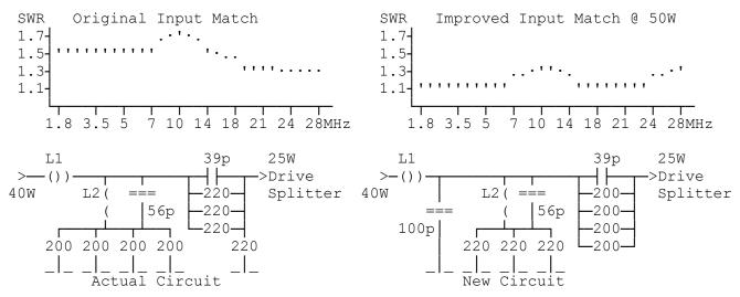
There was a bump @ 10MHz & that is from the drive splitter load. L2 & 56pF disconnects the added load, as the 39pF bypasses the series attenuator Rs on the higher frequencies, to flatten the amp gain. The original diagram did not have 220R to ground, but had 20pF to ground @ the L1/2 junction. I found making this a 100pF (Tx grade) was better on 10m band & changing the load Rs around gave a better lower band input match.
