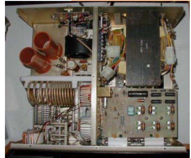
Photo 3. The innards. Rear panel at top, front panel at bottom. The 8874s live in the top left compartment. The Pi-L network is at the lower left. The RELAY jack is at top center, near the power transformer. The High Voltage & Control PCB covers the lower right quadrant.
