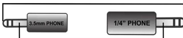
Figure 15. CW Key Tune Cable. Use stereo (TRS) plugs as shown, mono plugs may short adjacent terminals.
