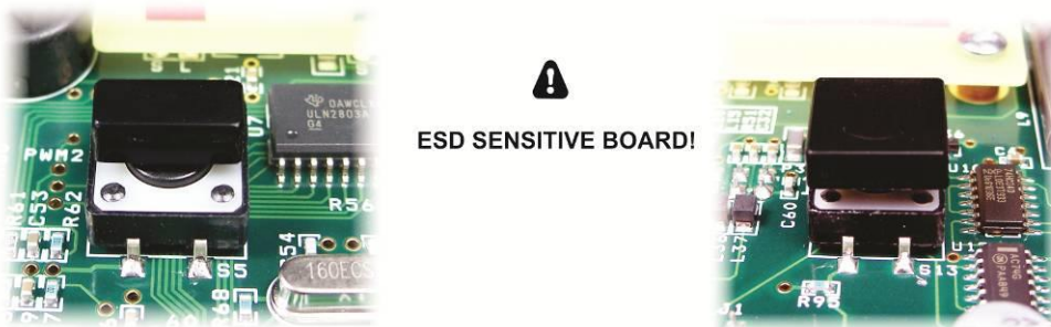
Figure 57. Installing Key Caps on Front Panel Board.
