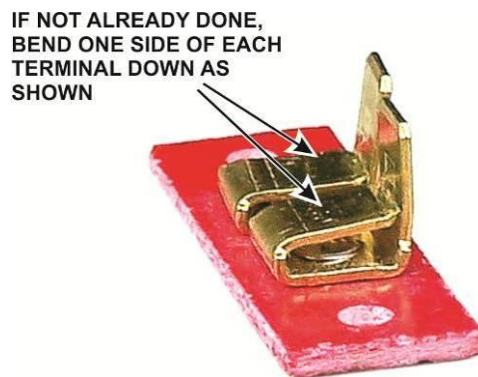
Figure 17. Preparing the Terminal Strip Board.
