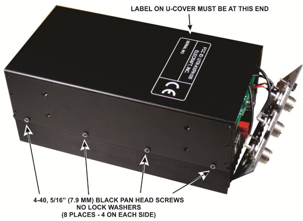
Figure 19. Mounting the U-Cover.
