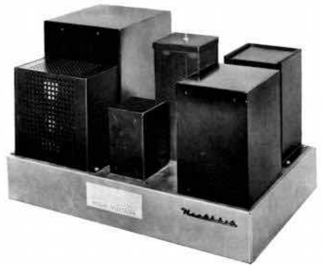
Figure 1: Heathkit KS-1 3,000 V Power Supply with its open frame construction. Rectifier tubes (A pair of 866A's) are in meshed cage at front left.
