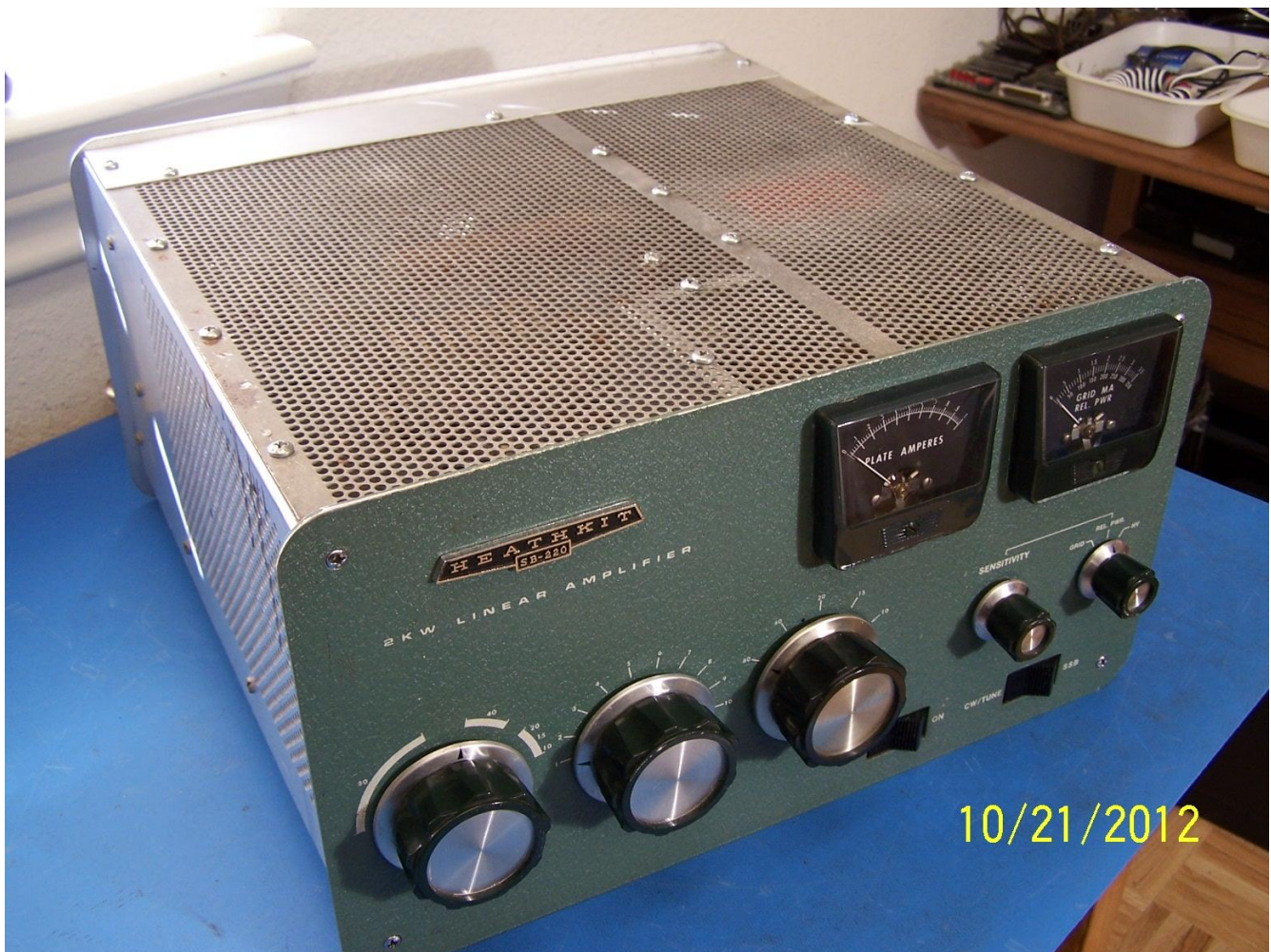
Photo 1. The Heath SB-220 at the beginning of the project. The outer enclosure has been removed.
