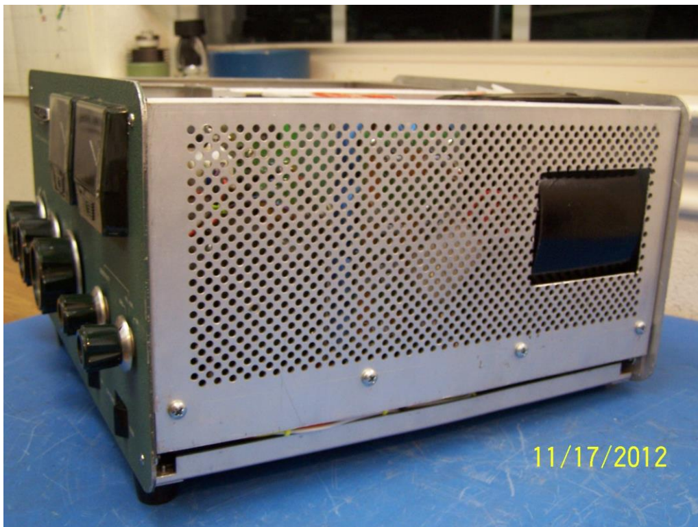
Photo 12. It was necessary to cut a rectangular hole in the right-side panel to make room for the Harbach transformer. The transformer will not interfere with the outer enclosure for the amp.
