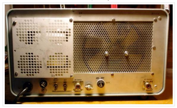
Since the CW/SSB switch became redundant, I changed the circuitry so that it is a Standby/Operate switch that kills the HV. (Yes, I know it's not needed as the 3-500s are instant on, but it's better than leaving it there doing nothing.)
