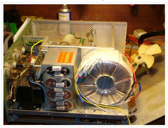
I ordered the 800 VA one as it would just fit in the cavity. It's specs were 2 x 650 VAC secondaries and 2 x 115 VAC primaries. Our mains voltage here in ZL is 230VAC and the amp has long been converted to that. And the cost was \$99.00 – about one third the price of a Dahl replacement. I seriesed the two secondaries for 1300VAC and the SB220 brought them up to 2600V x 1.41 which gave me 3600 VDC on the 3-500s. A bit high, but liveable.
