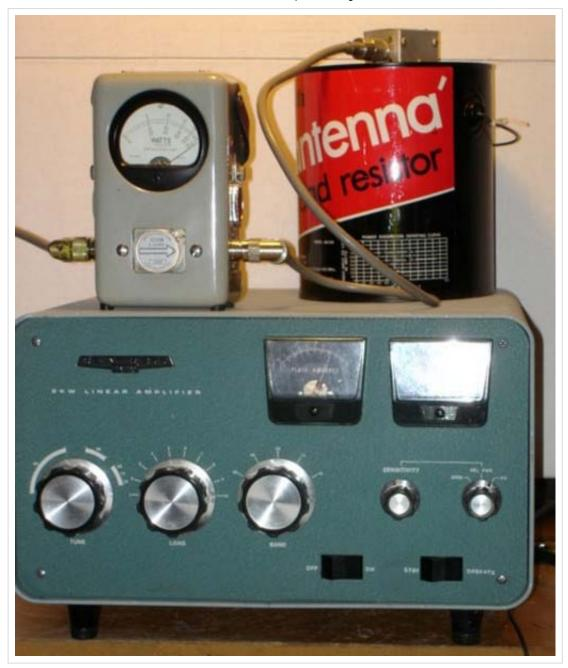
It will actually put about 1400 watts into the antenna but that it a long way past the capabilities of the band switch and variable capacitors so running it at around 900 to 1000 watts seems to sit well with it.
