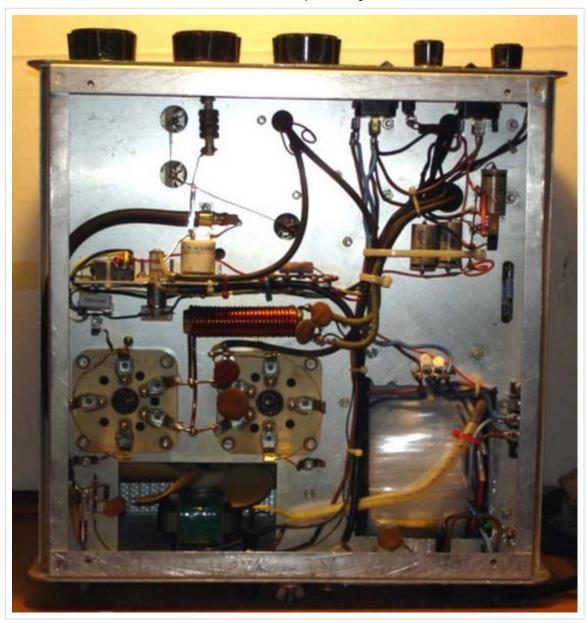
2) Remove the antenna switching relay, mount it near the circuit breakers and rewire it as a "Step Start" relay to bring the voltage up on the filter capacitors slowly, limiting inrush current and protecting the main power switch along with the power supply components.
