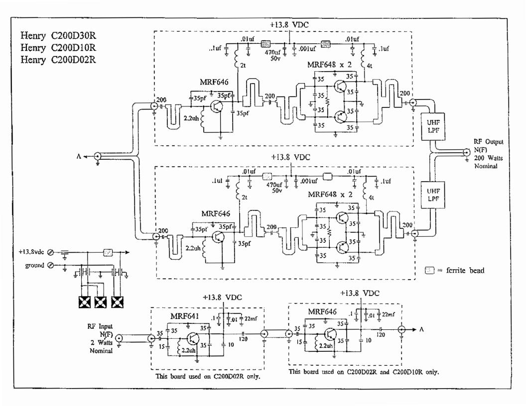
NOTE; SOME COMPONENTS AND WIRING OMITTED FOR CLARITY.
