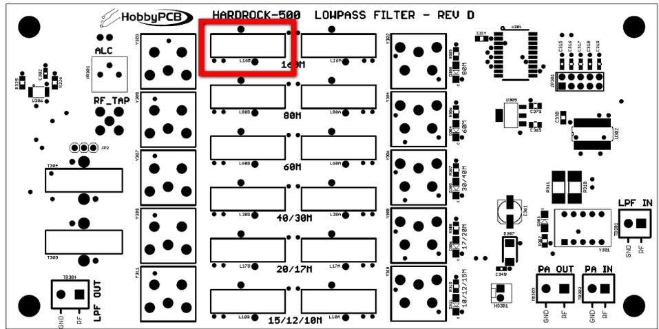
□ **Step 13: T303/T304** – 30 turns (30 in/76.2cm) of #28 enameled wire on a T82-43 (gray) toroid core. Wind the inductor, scrape and tin the leads and then insert the inductor into the PCB at the marked location. Solder and trim the excess leads. *Two of these coils are required T303 and T304 as shown*
