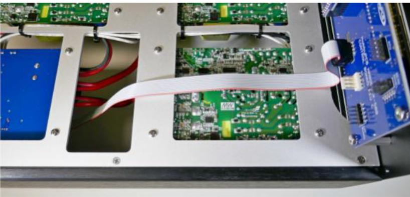
Turn the assembly on its side and connect the other end of the cable to the 10 pin header on the power board. Make sure that the pins align correctly and the cable is flat with no twists.
