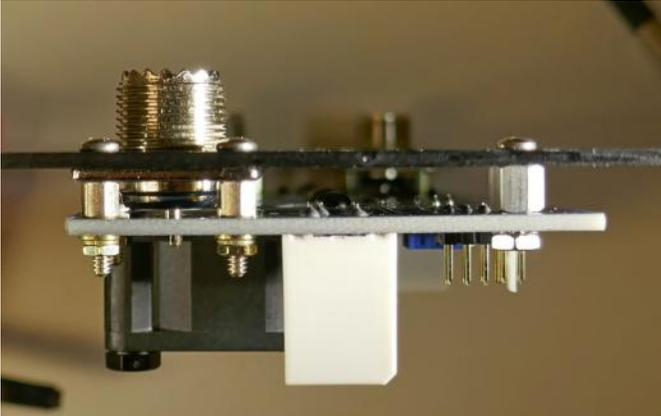
□ **Step 7: SO239 screws** – Use the thirteen #4-40x1/4” screws to fasten the SO239 jacks and the 1/4” spacer to the rear panel. Then solder the center pins of the SO239 jacks.
