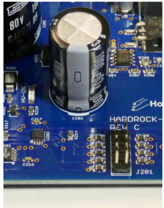
**Step 3: Check Capacitor Polarity** –Review the pictures and your PCB one more time to make 100% certain that C201 and C206 are oriented correctly. Solder them to the PCB and trim any excess leads.
