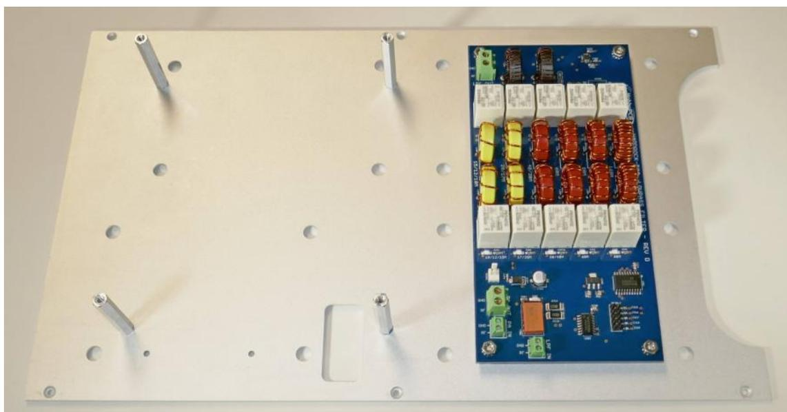
□ **Step 20: Side Panels** – Get two of the extruded side panels and use 6 #4-40x $\frac{1}{4}$ ” flat head screws to attach the side panels to the top of the RF Deck Panel, use thread-locker if available. *In run 1 of the amp the counter sink is on the wrong side of the panel. In this case there is plenty of clearance for the flat head screws and we decided to assemble the amps using the panels as built. The screws are not visible once the amp is assembled.*
