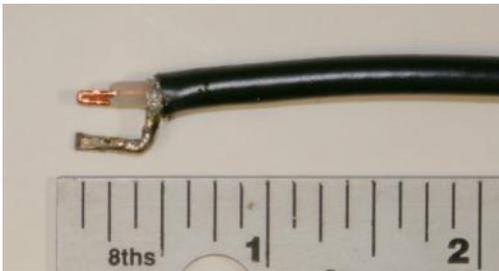
**Step 20: Amp In RF Jumper** – Cut a 9” (23cm) piece of RG-58 coax and prepare the ends in the same manner.
