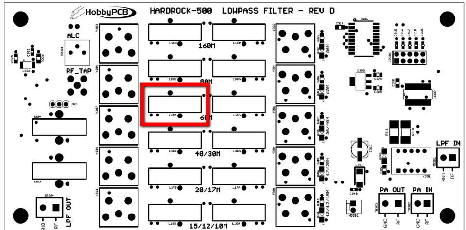
□ **Step 10: L80A** – 17 turns (18 in/45.7cm) of #20 enameled wire on a T80-2 (red) toroid core. Wind the inductor, scrape and tin the leads and then insert the inductor into the PCB at the marked location. Solder and trim the excess leads.
