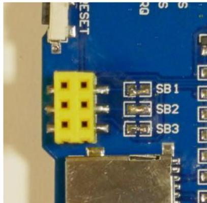
Use a component lead or small piece of wire to solder across the space between the pads of SB1, SB2 and SB3 as shown. For those not intimidated by SMT components, low value resistors will work fine and are easier (I think) to deal with than the jumper wires. Any resistor less than 100 ohms will be sufficient.
