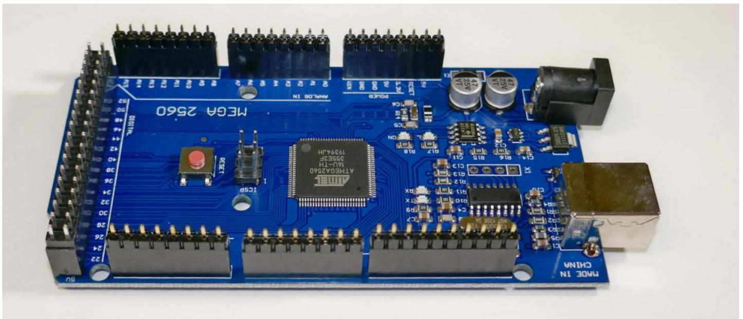
**Step 8: Mount Mega on PCB** – Insert the short pins into the front panel PCB on the opposite side from the LCDs, it's labeled “INSTALL ARDUINO MEGA ON THIS SIDE”.
