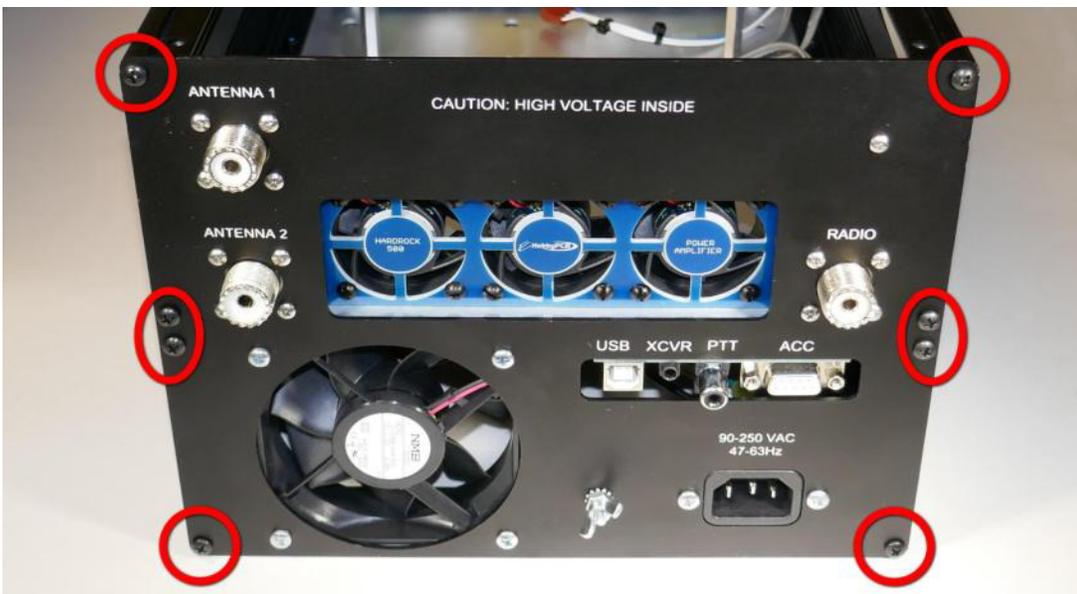
□ **Step 8: AC Inlet Wires** – For safety be sure to make the correct AC line, neutral and ground connection to the AC power inlet. Looking into the connector side of the AC inlet from the rear panel are the locations of the (G)round, (L)ine and (N)eutral AC connections.
