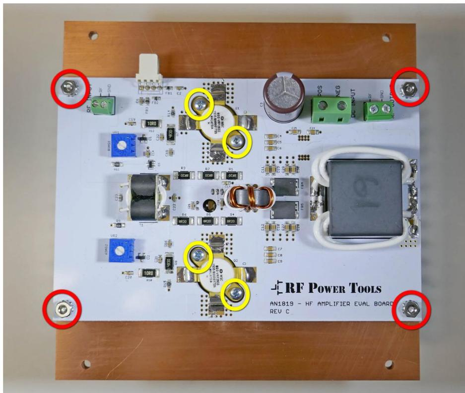
Turn the BIAS1 and BIAS2 potentiometers fully counter-clockwise (CCW).
