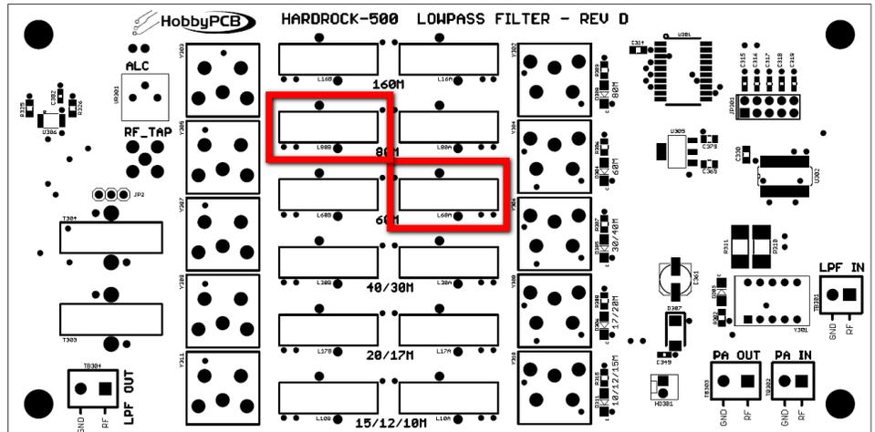
□ **Step 9: L60B** – 15 turns (16 in/40.6cm) of #20 enameled wire on a T80-2 (red) toroid core. Wind the inductor, scrape and tin the leads and then insert the inductor into the PCB at the marked location. Solder and trim the excess leads.
