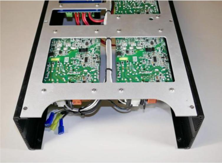
**Step 2: Front Panel**– Attach the front panel to the power supply assembly using four #6-32 3/8” black, pan head screws. *Do not completely tighten the screws at this time.*
