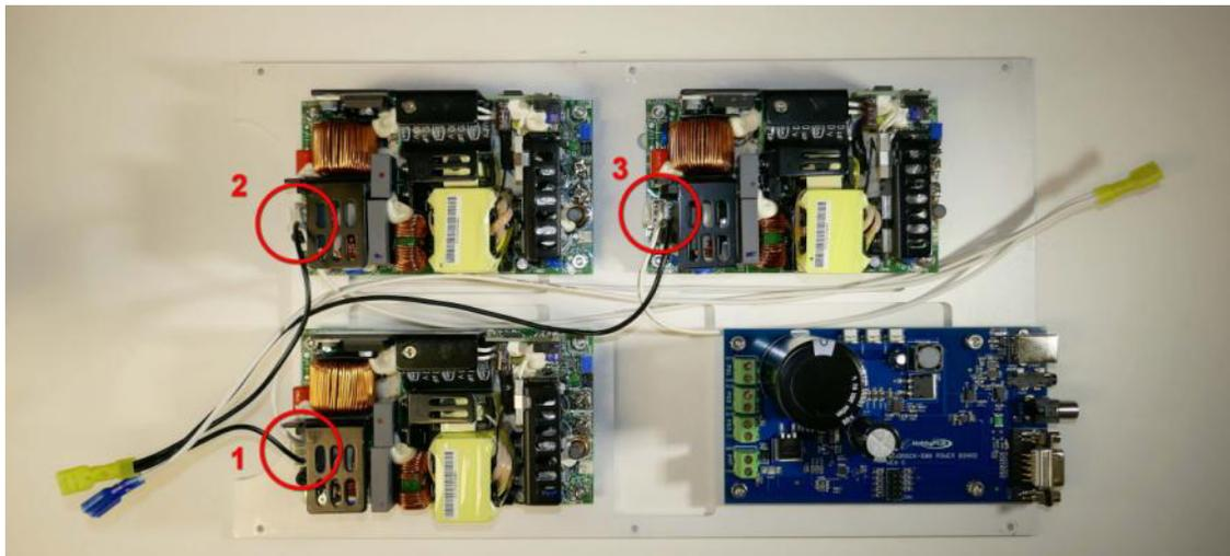
□ **Step 11: AC Switch Wire** – The AC Switch wire is a single conductor with blue crimp terminals on either end. Place it with one end near each of the yellow crimp terminals. No connections are made at this time.
