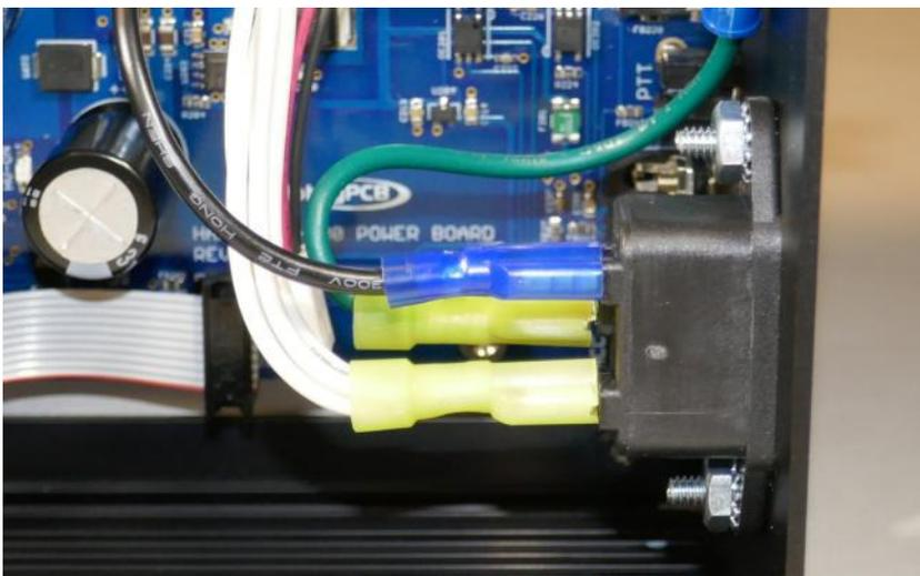
□ **Step 9: 80mm Fan Wire** – Plug the wire from the 80mm fan into the fan connection of the closest Meanwell power supply. If there is any excess wire, wrap it up neatly. The black wire is towards the DC connections.
