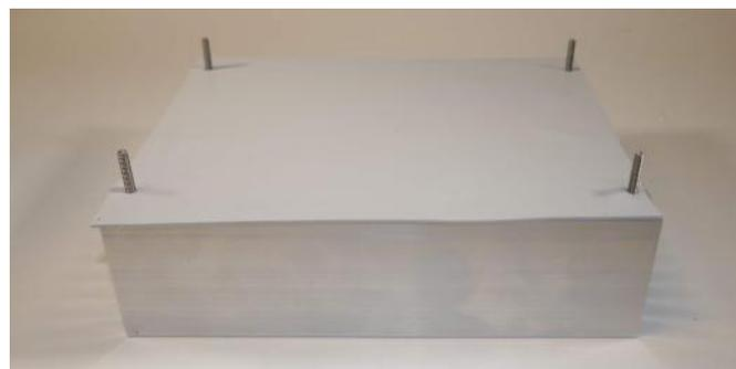
□ **Step 24: Copper Heat Spreader** – The copper heat spreader is not symmetrical and needs to line up with the holes in the heatsink. Unfortunately, with the thermal pad covering the heatsink, you cannot determine where the holes in the heatsink are. Make sure that you have the right side up:
