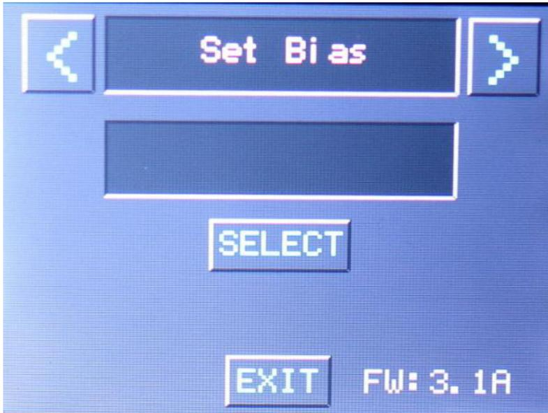
*Check to make sure that both BIAS pots on the AN-1819 board are fully counter-clockwise (CCW). Turning the bias on in the next step can damage the VRF2933 MOSFETs if the BIAS pots are not fully CCW.*
