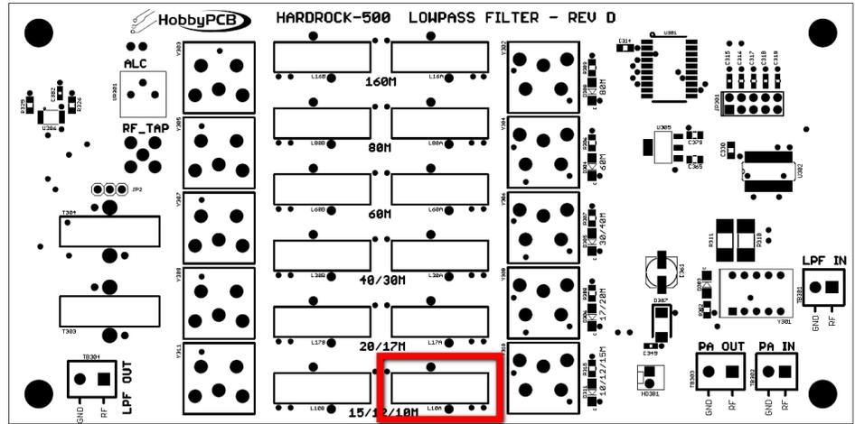
□ **Step 3: L10B** – 5 turns (7 in/17.8cm) of #20 enameled wire on a T80-6 (yellow) toroid core. Wind the inductor, scrape and tin the leads and then insert the inductor into the PCB at the marked location. Solder and trim the excess leads.
