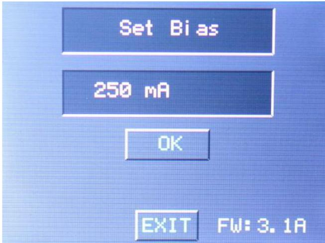
**Step 6: Adjust BIAS 2** – Slowly turn the BIAS2 pot on the AN1819 board until the current reaches an additional 250 mA above the setting obtained in step 5.
