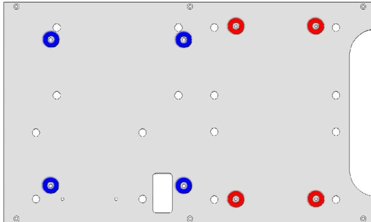
□ **Step 17: AMP Deck Hardware** – At the four locations indicated in blue, insert a #6-32x3/8" pan head screw from the opposite side the panel into a #6-32x1.75" F-F threaded stand-off. Tighten securely. Use thread-locker if available.
