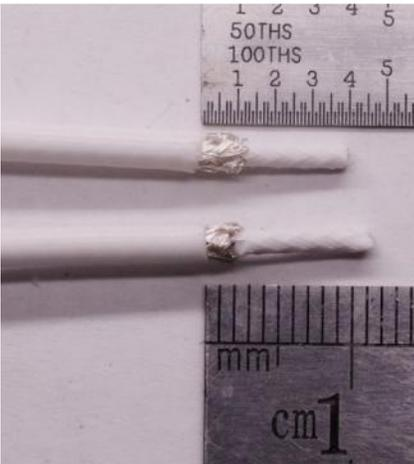
Strip 0.2” (6mm) of the dielectric and tin the shield and exposed center conductor (the outer jacket and dielectric are both Teflon that doesn't melt).
