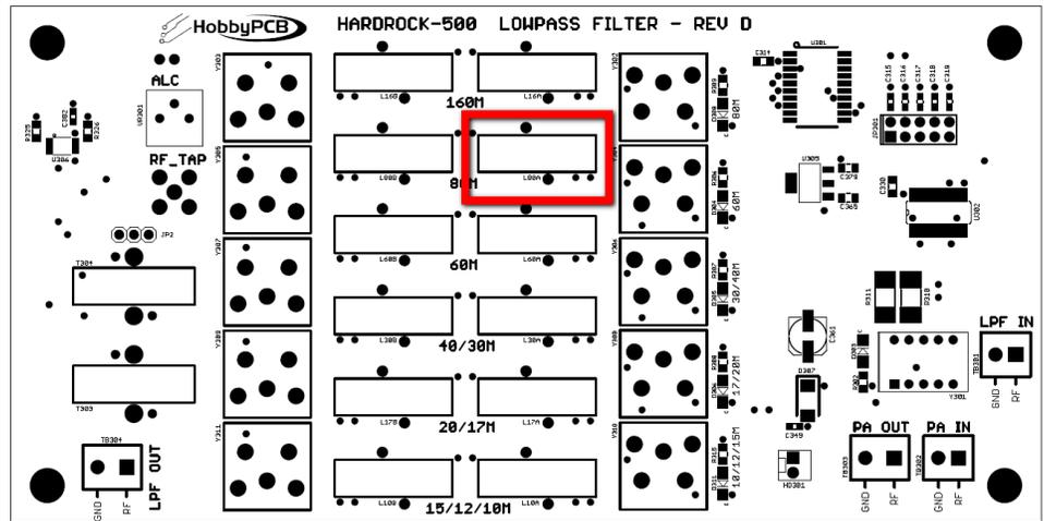
□ **Step 11: L16A** – 20 turns (20 in/50.8cm) of #20 enameled wire on a T80-2 (red) toroid core. Wind the inductor, scrape and tin the leads and then insert the inductor into the PCB at the marked location. Solder and trim the excess leads.
