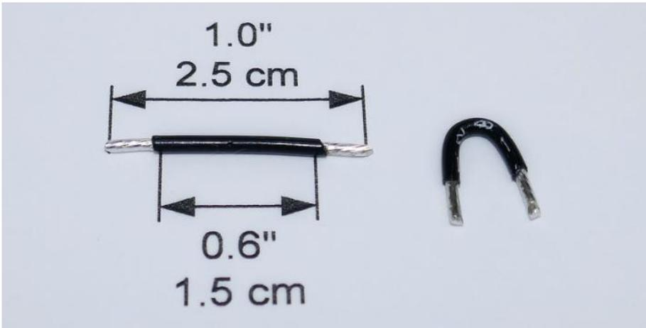
□ **Step 15: T303/T304** – insert the #18 wire ‘U’ created in step 14 through T303 and T304 into the larger diameter holes on either side of the cores. Solder the ‘U’ wires in place and trim excess leads. *Note JP2 is shown installed for normal operation.*
