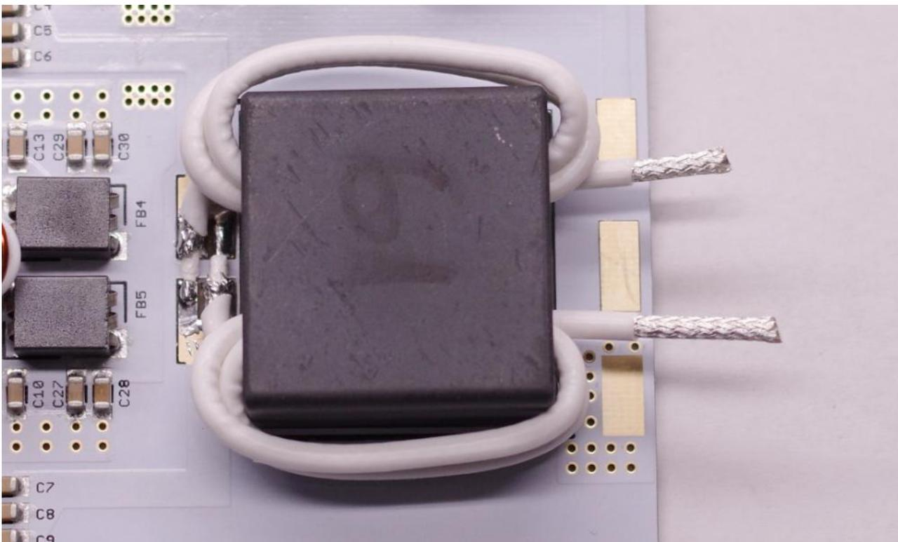
Strip the outer jacket of the protruding coax to approximately ¼” (6mm) from the core. Carefully unbraid the shield wires and gather them towards the center of the three pads on the edge of the circuit board. Strip the dielectric from the center conductors.
