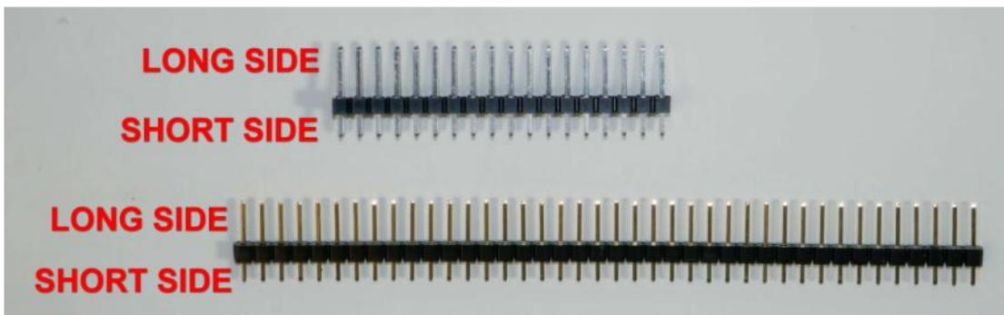
□ **Step 7: Insert Pins** – Insert the dual header into the dual row receptacle on the Arduino Mega. Use the 40 pin single row headers and break off the appropriate number of pins for each of the single row receptacles on the Arduino Mega. Make sure that every connection on the Mega has a header pin.
