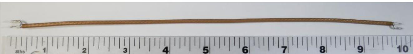
**Step 18: Amp In RF Jumper** – Cut a 5” (13cm) piece of RG-316 coax and prepare the ends in the same manner.
