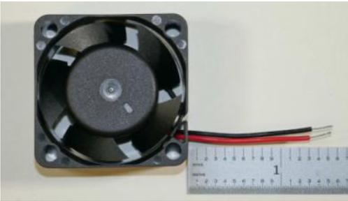
□ **Step 2: Mount Fans** – Mount the three fans to the rear panel board using 12, #6-32 1" black nylon screws and 12, #6 black nylon nuts. Orient the wires as shown (towards the top of the PCB and the label on the fan should be against the PCB). *The mounting hardware is nylon plastic. Tighten them snugly but do not over-tighten to avoid breaking the screws.*
