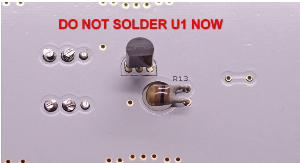
Solder R13 and trim the excess leads. **DO NOT SOLDER U1 NOW.** The AN-1918 is now ready to be mounted on a suitable heatsink.
