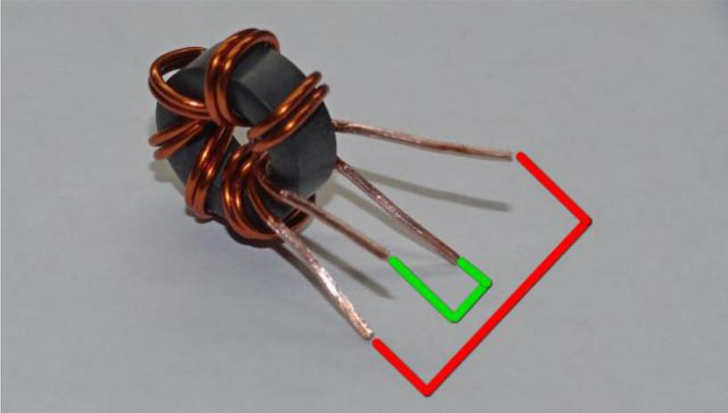
**Step 6: Install T2** – Once you have the leads aligned correctly, insert the leads of T2 into the PCB. The enameled wires are inserted into the larger holes in the footprint
