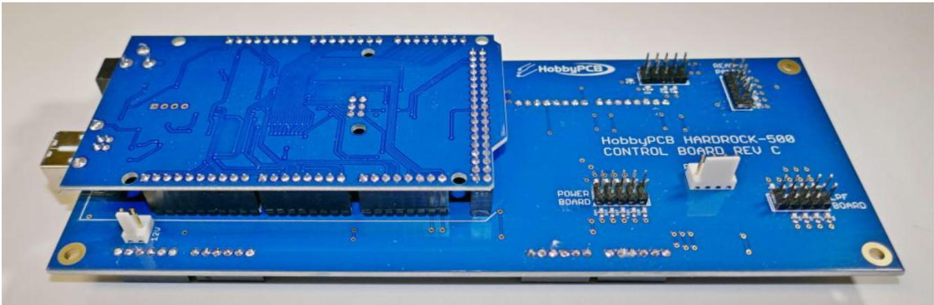
**Step 9: Solder Mega Pins** – Carefully solder the pins on the opposite side of the PCB from the Arduino Mega. Be sure that the Mega is flush with the PCB. Use as little solder as possible. Just fill the plated through holes with solder. There is no need for a large amount of solder to accumulate on top of the board and there is no need to trim the pins on the Mega.
