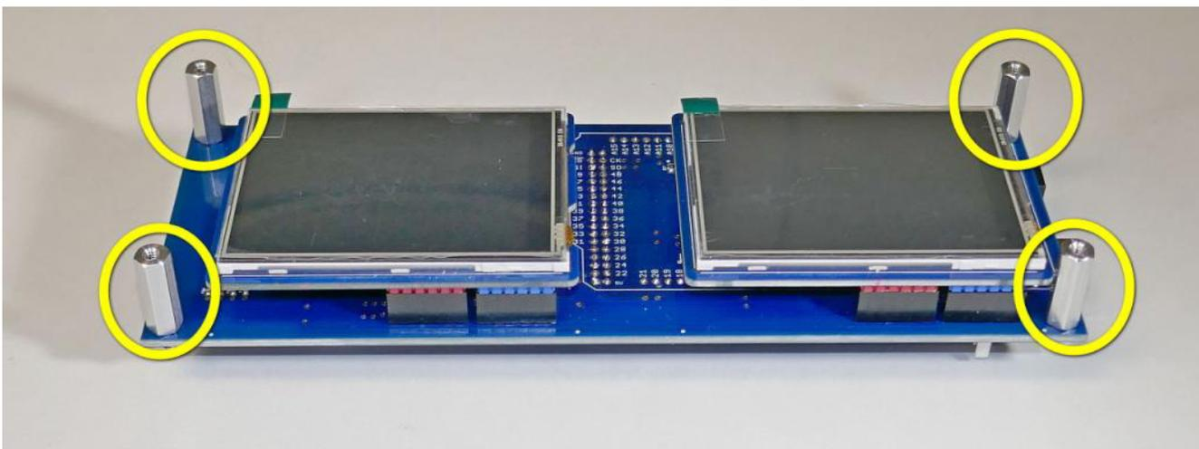
□ **Step 12: Front Panel** – Remove the protective film from the front of the LCDs (it’s not possible to do it after you mount the front panel PCB). There are two possible ways to mount the front panel PCB to the back of the front panel, only one of these causes the LCDs to align correctly with the openings. Orient the front panel board with the LCDs aligned with their openings. Use the #4-40x1/4” black screws to secure the PCB to the front panel.
