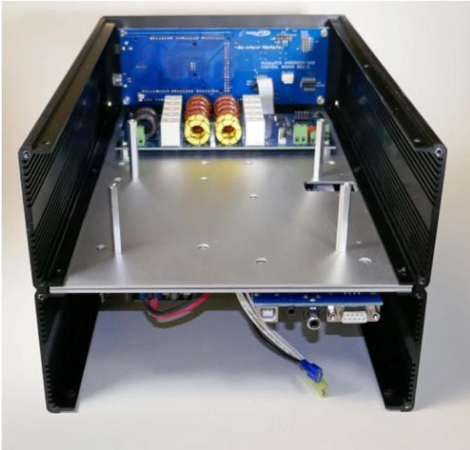
□ **Step 5: Front Panel** – Attach the front panel to the LPF assembly using four #6-32 3/8” black, pan head screws. Tighten all front panel screws.
