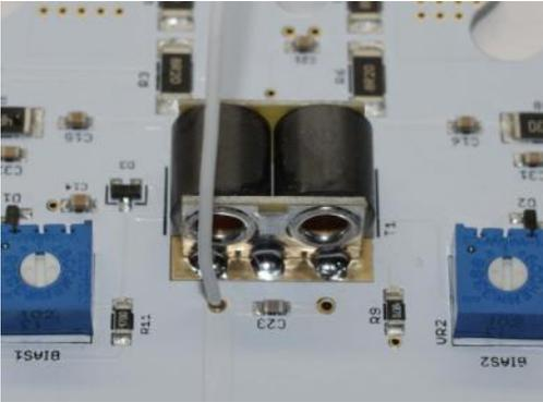
Pass the wire through the holes in the core, up and back a total of 3 times. Trim the wire, strip off the insulation and solder the wire into the hole in the PCB on the other side of C23. Trim any excess wire flush with the PCB.
