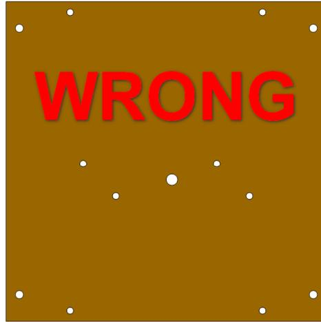
You can see the holes in the heatsink from the fin side and align the heat spreader correctly on the heatsink. If the alignment is correct, a screwdriver placed in the large hole near the center will pass through the heat spreader, through the thermal pad and through the heatsink. If it doesn't, turn the heat spreader around.
