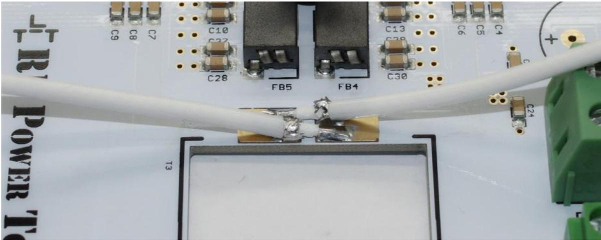
□ **Step 10: Wind T3** – Place the rectangular core into the opening in the PCB with the holes in the core adjacent to the coax sections. Pass the coax pieces through the holes in the core then around the outside of the core and through the hole again a total of three passes through the core.
