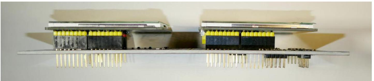
**Step 4: Solder/Check LCDs** – Start by placing the assembly on a flat surface and soldering a single pin on either side of each LCD then press down on the PCB close to the pin to ensure that the header is fully seated. Then check the alignment. It is critical that the headers are fully seated, flush with the PCB and perpendicular to the PCB.
