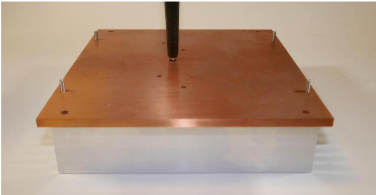
□ **Step 25: Nylon Washers** – Place one #4 nylon washers on each of the threaded rods, (the washer in the kits may be black). Put a small amount of heatsink compound in the large hole in the center of the heat spreader.
