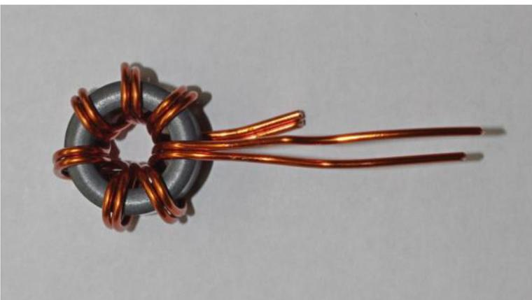
*Remember all of the DC current for the amplifier passes through these windings on T2, make sure to remove all of the enamel and tin the wire completely.*
