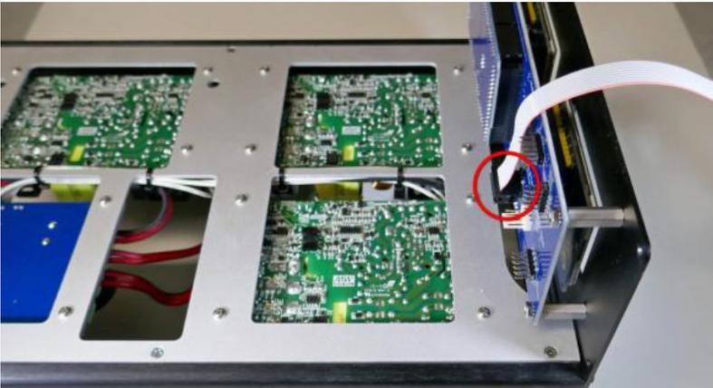
Bend the ribbon cable back across the connector and route the cable through the rectangular opening in the power supply plate as shown. Make sure that the cable is flat and not twisted. The polarity indicator on the cable can be on either side.
