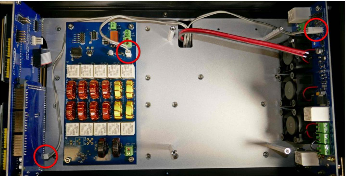
□ **Step 15: Short Ribbon Cable** – Connect the short ribbon cable (3” or 8cm) to the front panel board and the LPF board. Make sure that the alignment is correct and the cable has no twists.
