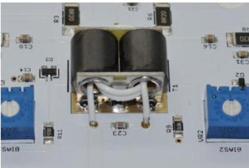
You should see two wire loops on this end of the core and three loops on the other end of the core.
