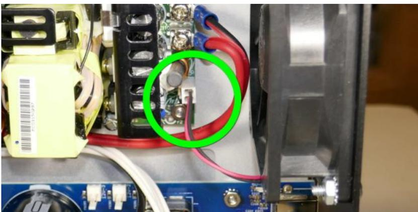
□ **Step 10: Amp Power Wire** – Insert the remaining #14 red/black zip wire (6” long with no terminals) into the AMP terminal block on the power board and tighten the screws. Route the free end of the wire through the rectangular hole adjacent to the power board.
