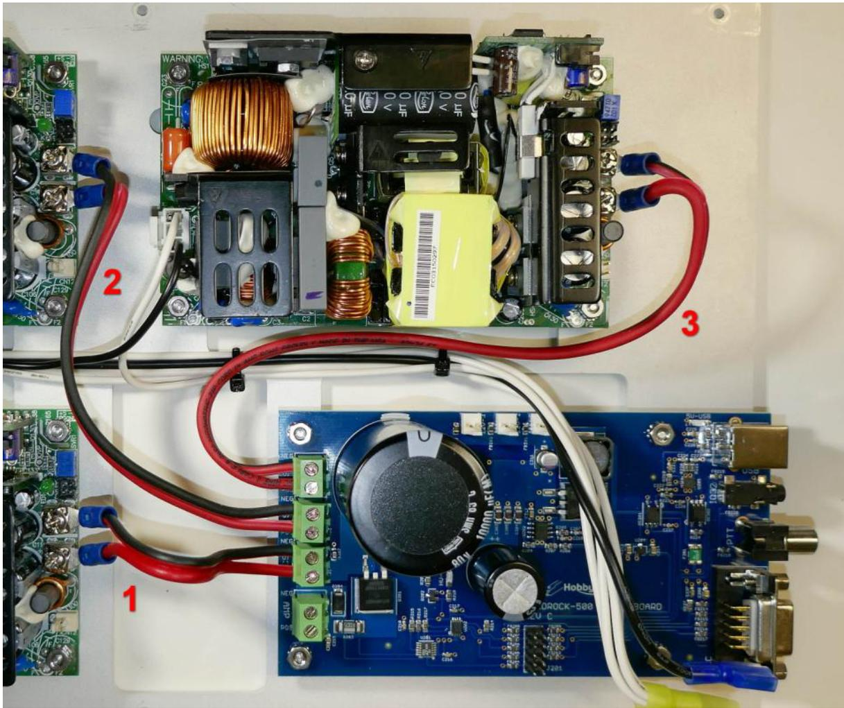
*Leave the 'AMP' terminals on the power board unconnected at this time.*
