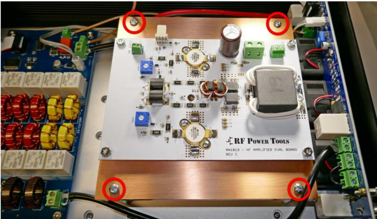
**Step 29: Amplifier Cables** – Connect the RF Input (green), DC Input (red), and RF Output (yellow) cables. Be sure that the ground and RF connections are correct on the RF connections and the polarity is correct on the DC cable (red is positive, black is negative).
