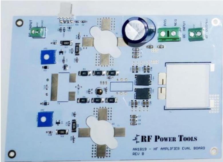
**Step 1: Trim Leads** – Carefully trim the leads of the terminal blocks, VR1 and VR2 so that no more than 0.1” (.25cm) projects from the bottom of the PCB. *The PCB mounts VERY close to the copper heat spreader so it is important to cut all leads on the bottom of the board as close as possible to prevent shorts.*
