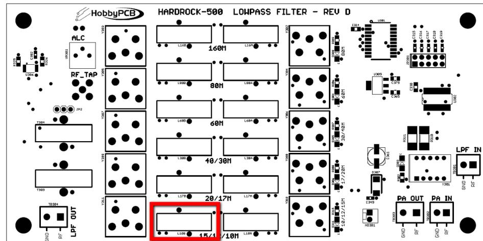
□ **Step 8: L60A & L80B** – 16 turns (17 in/43.2cm) of #20 enameled wire on a T80-2 (red) toroid core. Wind the inductor, scrape and tin the leads and then insert the inductor into the PCB at the marked location. Solder and trim the excess leads. *Two of these coils are required for L60A and L80B as shown*
