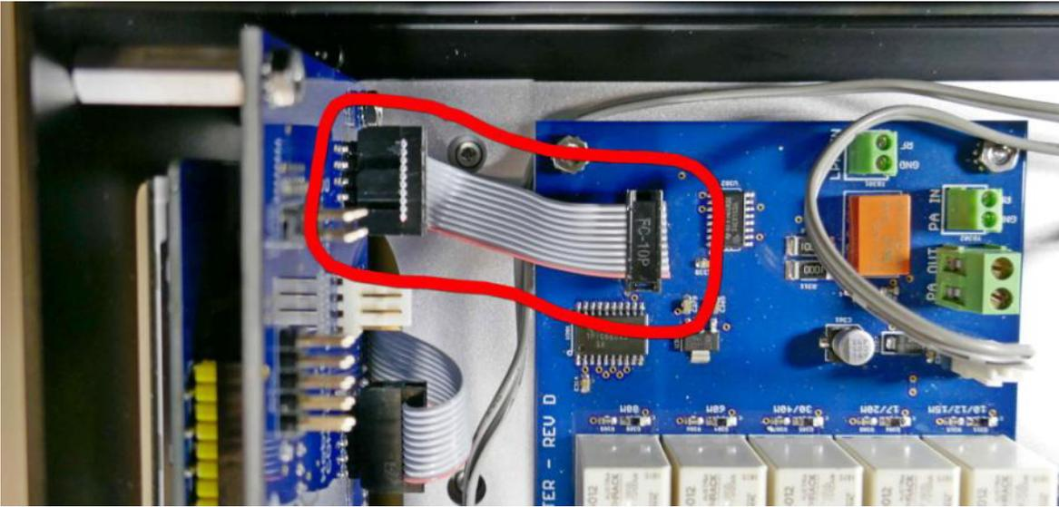
□ **Step 16: Long Ribbon Cable** – Connect the long ribbon cable (14” or 35cm) to the front panel board and the rear panel board. Make sure that the alignment is correct and the cable has no twists.
