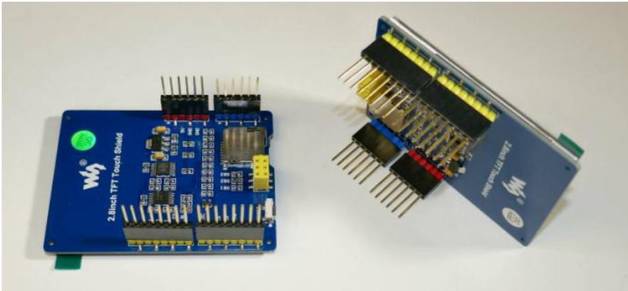
**Step 3: Mount LCDs** – On the side of the front panel PCB that says “INSTALL LCD DISPLAYS ON THIS SIDE”, insert the LCDs with the stacking headers attached. It’s a bit of a challenge to get all of the pins lined up.
