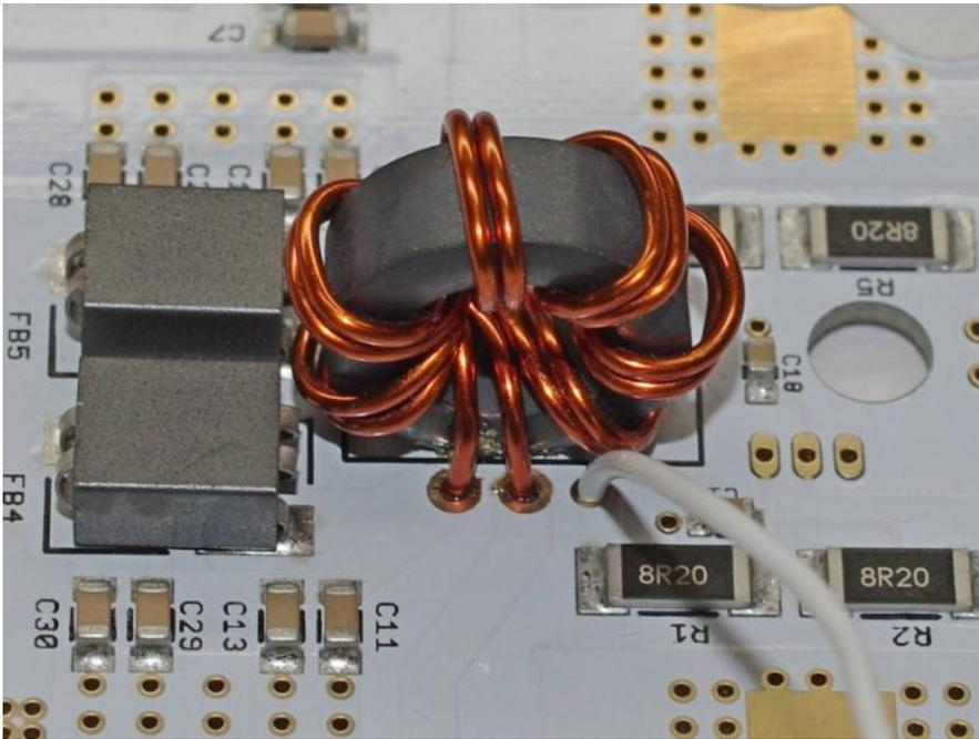
Wind the Teflon wire around T2’s core passing it through the core a total of three times.
