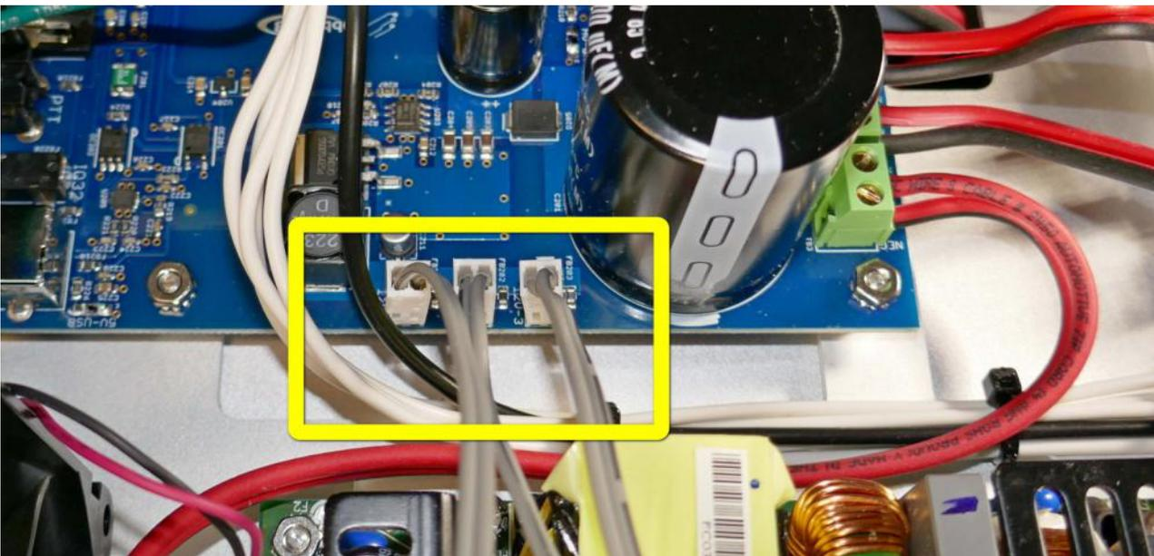
□ **Step 12: Route 12V cables** – Route the other ends of the 12V cables in a bundle, under the #14 red/black wires through the rectangular opening adjacent to the power board.
