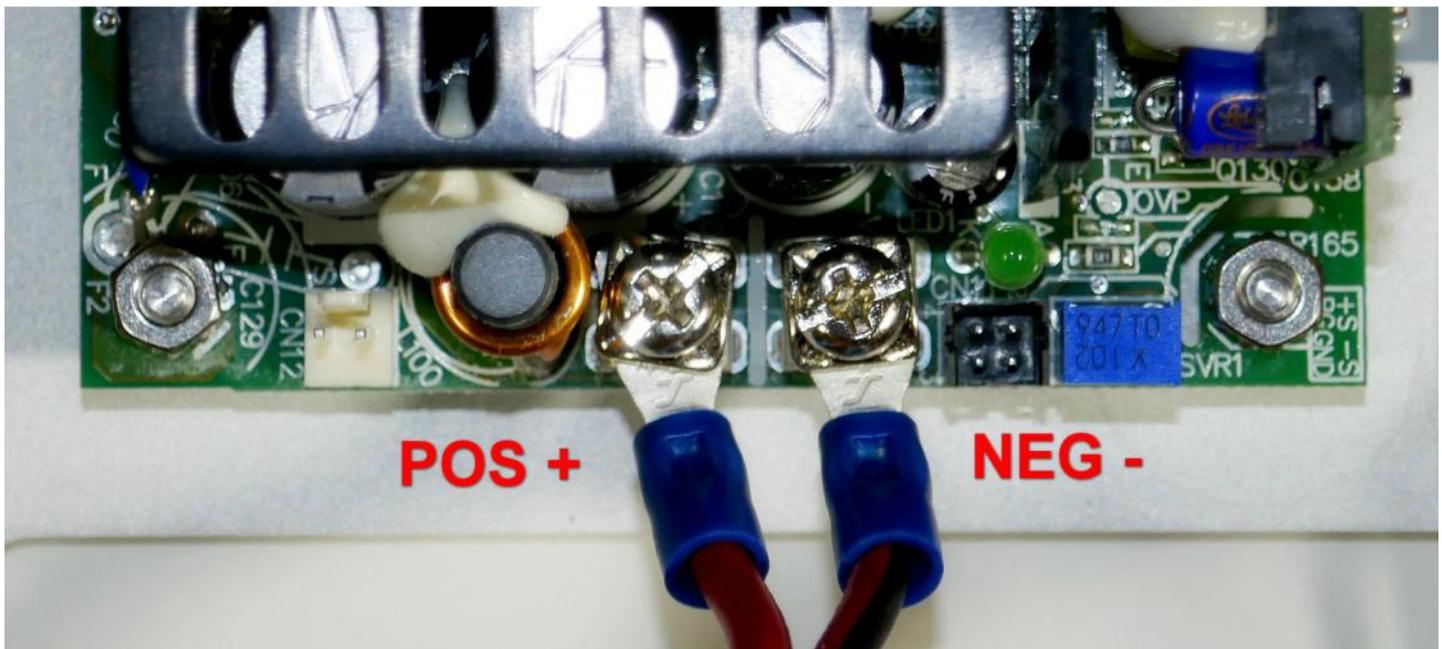
**Step 13: Power Board Terminal Blocks** – Loosen the screws in the terminal blocks on the power board by turning the screws CCW until you hear a click.
