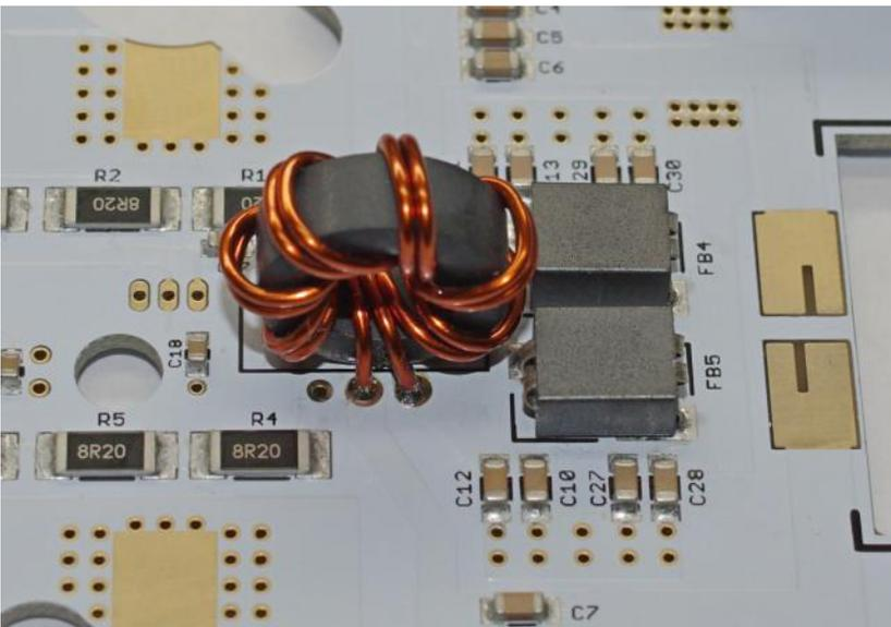
If these windings are correct, the drain tabs of Q1 and Q2 (indicated by a 'D' on the PCB) should conduct with the positive DC input. Once you have verified that this is correct solder leads of T2 to the PCB and closely trim the leads, there is very little clearance between the PCB and the heat spreader.
