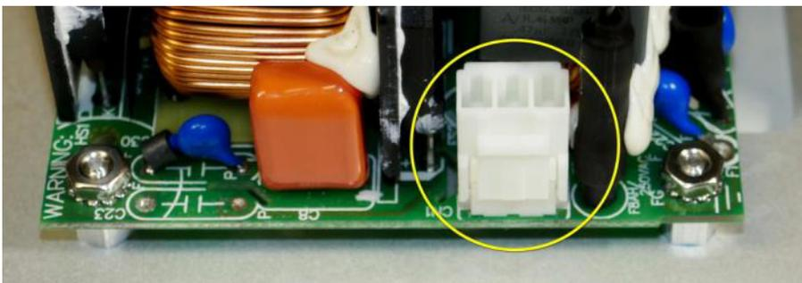
This is a drawing of the Meanwell EPP400-18 power supply we are now going to make connections to: CN1 Pin 1 – AC Neutral and CN1 Pin 3 – AC Line. Use needle nose pliers to insert the pins. The locking tab faces away from the edge of the power supply, towards the heatsink.
