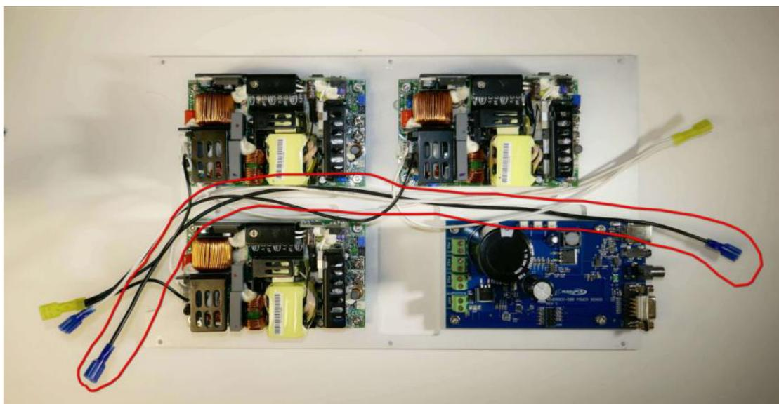
**Step 12: Secure AC Wiring** – secure the wire bundle to the power supply plate with four cable ties. *Make sure that the locking clip is on the wire side on the plate NOT below the plate or the two plates will not fit together.*
