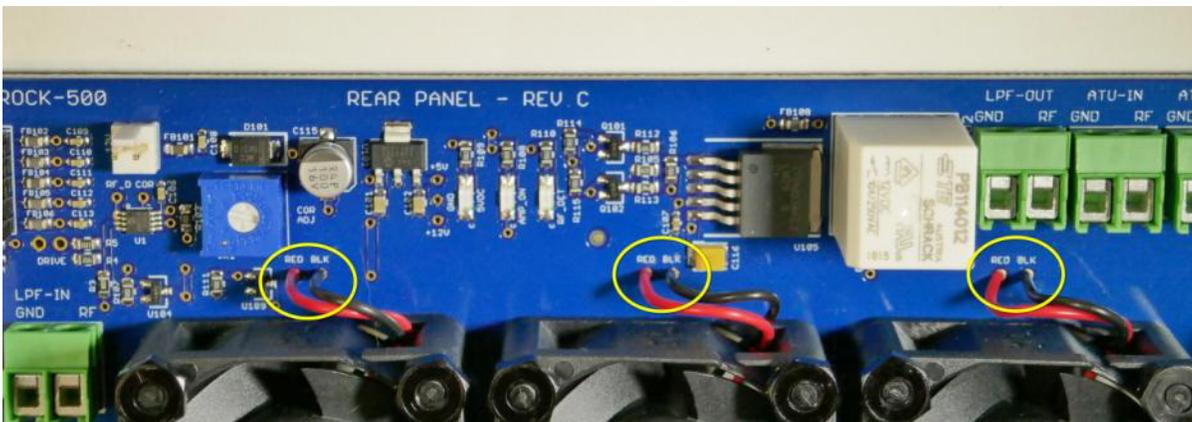
□ **Step 4: ATU Jumper** – Cut a 1.25” (32mm) section of #18 Teflon wire (from LPF board Step #14) strip the ends and create a jumper from the RF pin of ATU-IN to the RF pin of ATU-OUT. Tighten the screws in the terminal blocks.
