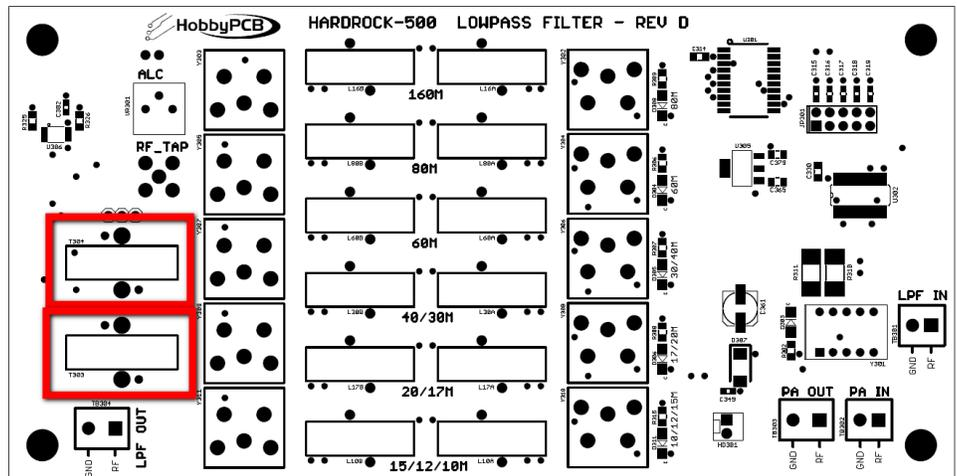
*T303 and T304 each have four holes in the PCB for wires. Be sure to insert the #28 wire in the holes with the smaller diameter. The larger holes will be used in the next steps.*
