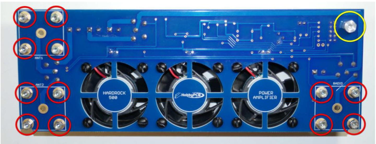
□ **Step 6: SO239 Mounting** – Place the three SO239 jacks over the jack screws with the center pins projecting through the PCB then place the rear panel over the SO239 jacks.
