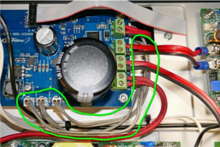
At this point the power supply section of the amplifier support kit is complete. Please compare your unit to the picture below to ensure that everything in this section is connected properly.
