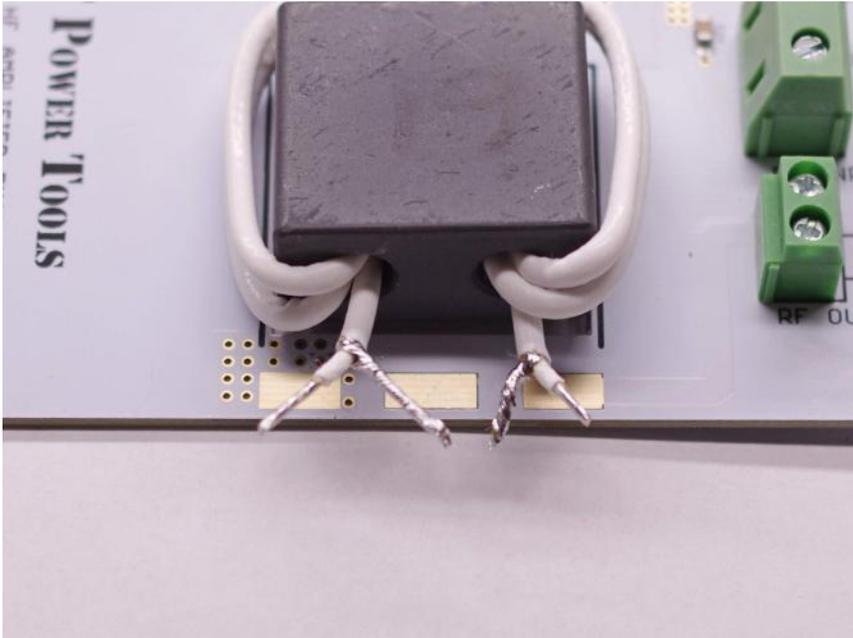
**Step 11: Complete T3** – Trim the wires and solder them to the pads. With each center conductor going to one of the outer pads and both shields going to the center pad.
