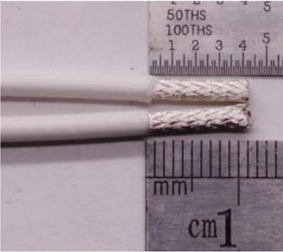
Cut the shield so about 0.1” (3mm) of the braid remains exposed.
