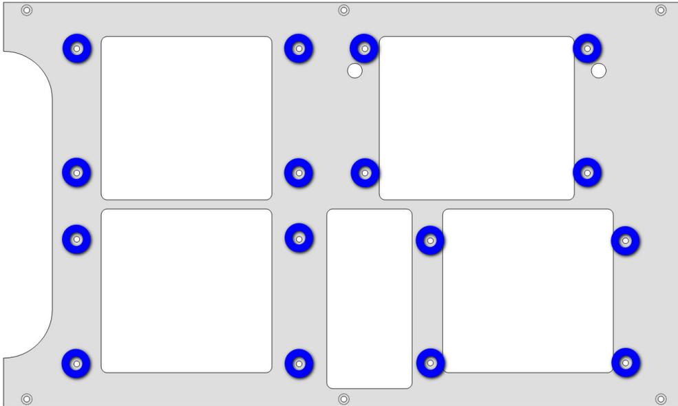
**Step 5: PCB Hardware** – At the sixteen locations indicated in blue, insert a #4-40x1/4" pan head screw from the opposite side the panel into a #4-40x1/4" M-F threaded aluminum spacer. Tighten securely. Use thread-locker if available.
