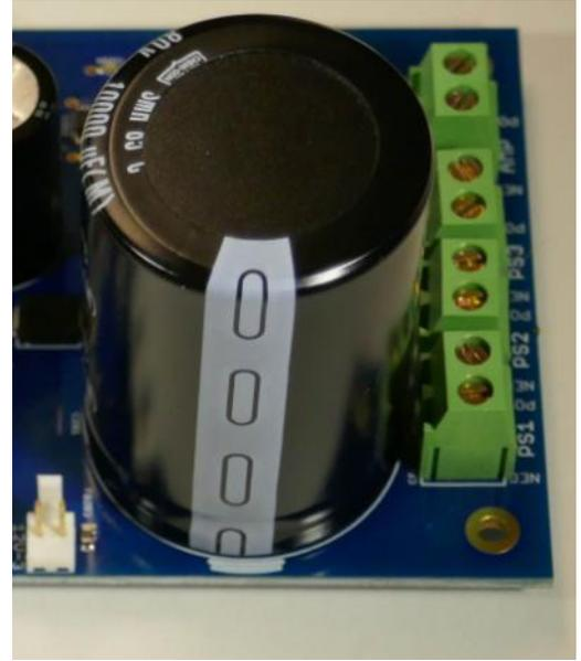
**Step 2: C206:** Insert C206, the 1000 uF, 63V, capacitor into the power board with the negative side of the cap closest to the 'C206' marking on the PCB. **DO NOT SOLDER AT THIS TIME.**
