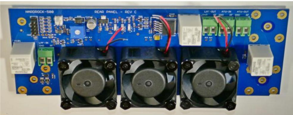
□ **Step 3: Connect Fans** – Insert the fan wires in the holes indicated on the rear panel board, solder the wires and trim any excess wire.
