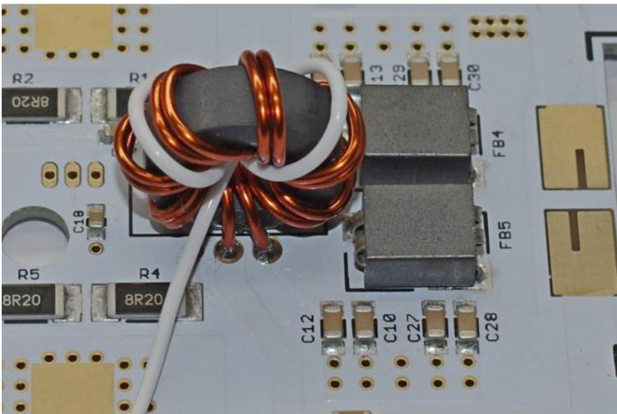
Cut the wire, strip the end and insert the wire into the remaining small hole in T2’s footprint. Solder the wire to the PCB and trim any excess flush with the PCB keeping in mind the limited distance between the bottom of the PCB and the heat spreader.
