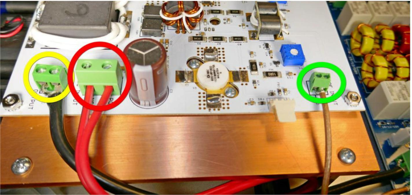
□ **Step 30: Amplifier Control Cable** – Connect four pin amplifier control cable between the front panel board and the AN1819 board.
