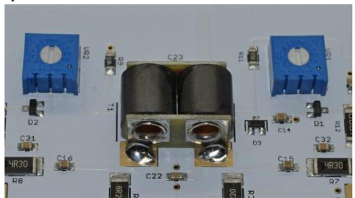
□ **Step 3: T1 Wind** – Cut an 8” (20cm) piece of #22 Teflon wire and strip ½” (1cm) of the insulation from one end of the wire. Insert the wire into the hole near C23 and R11 and solder the wire to the board and trim any excess wire flush with the PCB.
