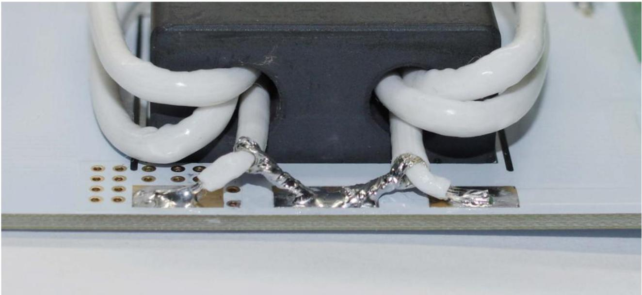
*The shield of this coax is NOT at ground potential. Do not touch the shield while the unit is operating and do not connect any portion of the shield to ground.*
