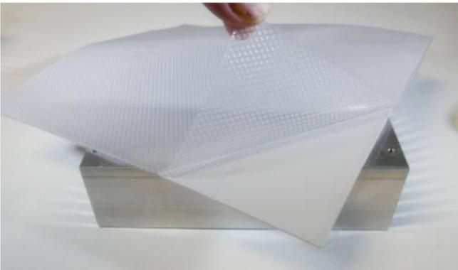
Line up one corner of the thermal pad with one corner of the heatsink and remove the other plastic sheet from the thermal pad. *The pad is 8" x 8" and the heatsink is only 4.6" x 6" so you will have some leftover thermal pad, save it, it may be useful in other projects.*
