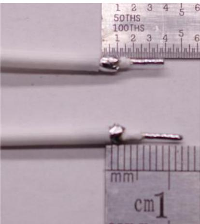
□ **Step 9: T3 Coax to PCB** – Solder the shield of one of the pieces of coax and the center conductor of the other to one of the pads of T3 on the PCB, repeat the process for the other shield and center conductor. The pad is split with wider side for the shield and the narrow side for the center conductor.
