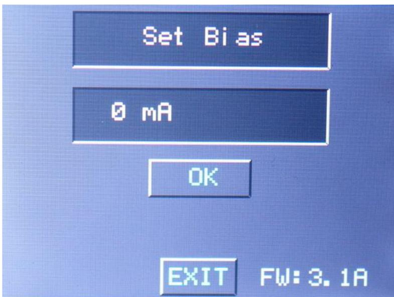
**Step 5: Adjust BIAS 1** – Slowly turn the BIAS1 pot on the AN1819 board until the current reaches 250 mA. Anywhere from 235 – 250 mA is acceptable. If it goes above 260 mA, turn it down.
