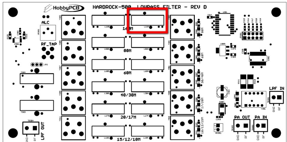
□ **Step 12: L16B** – 25 turns (25 in/63.5cm) of #20 enameled wire on a T80-2 (red) toroid core. Wind the inductor, scrape and tin the leads and then insert the inductor into the PCB at the marked location. Solder and trim the excess leads.
