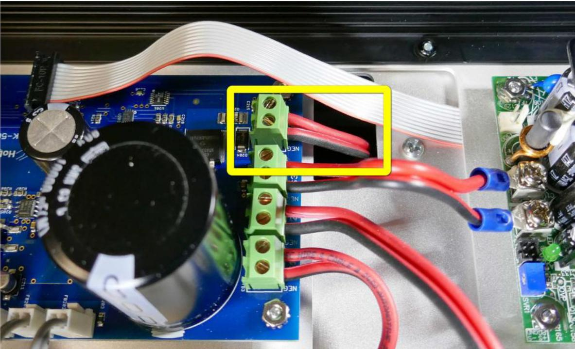
□ **Step 11: Connect 12V cables** – Plug the three 12V cables into the power board at the indicated locations. *The cables may be gray or red/black. All three locations are identical. The cables may be plugged into any 12V connector.*
