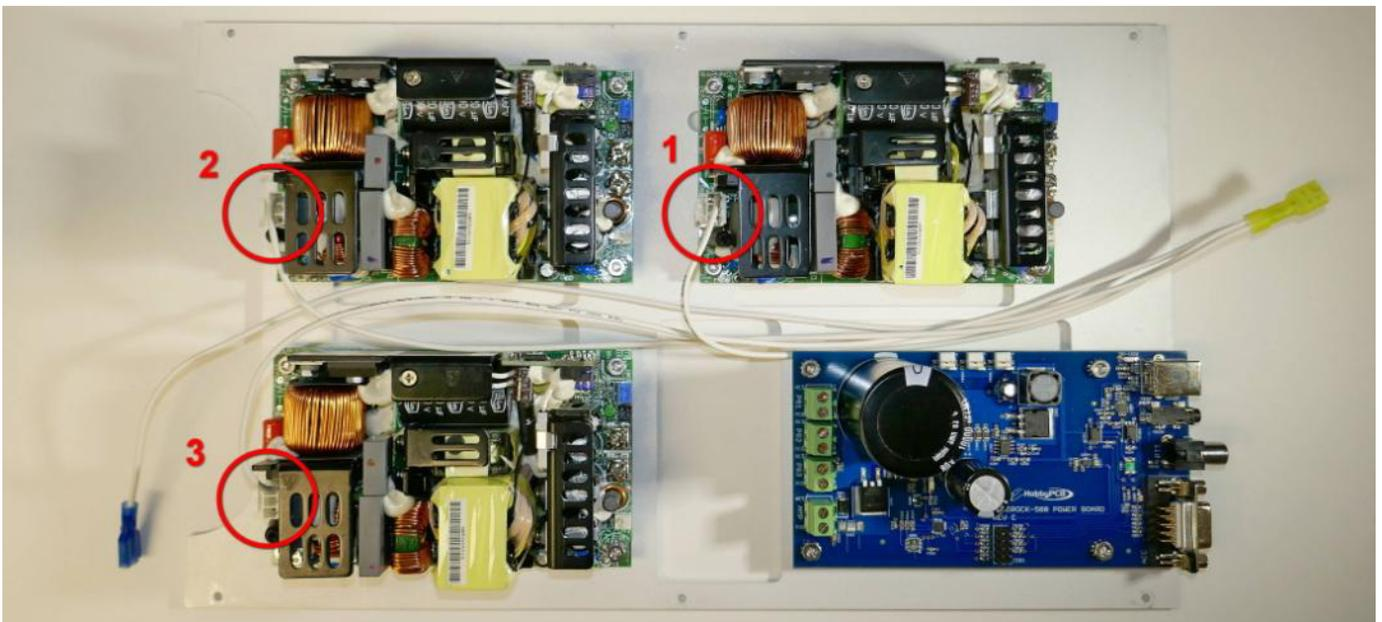
□ **Step 10: AC Line Wiring** – The AC Line Cable has three black wires with JST pins. The common end has a yellow crimp terminal, place this terminal at the left edge of the power supply plate.
