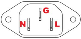
The ground connection should already be in place (chapter 12, step 9). Attach the AC line wire (blue terminal with a single black wire) and the AC neutral wire (yellow terminal with four white wires) to the appropriate connection point on the AC inlet.
