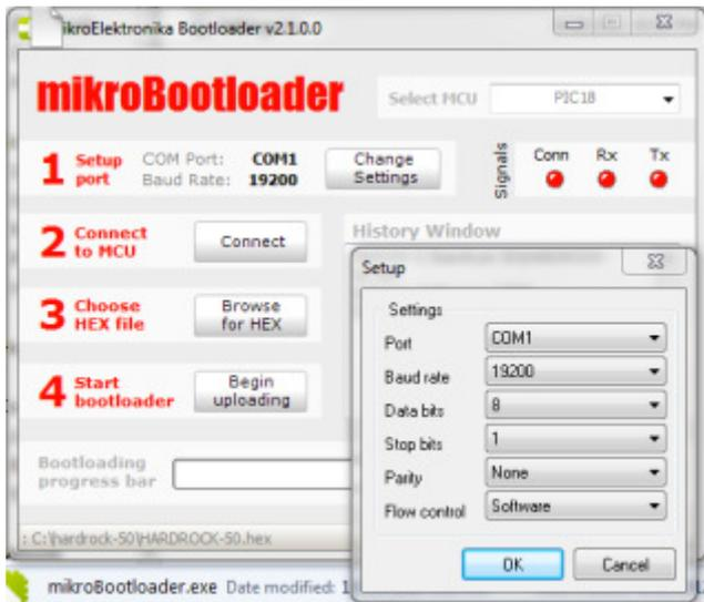
Change the Port to whatever COM port your HR50 registered as. Leave the rest of the settings alone and click OK. If you don't know which port your HR50 is on, start the bootloader with the HR50 powered off, note which ports are available. Shut down the bootloader, power up the HR50, restart the bootloader and the new port in the list will be the HR50's port. Make sure PIC18 is selected in the Select MCU box.
