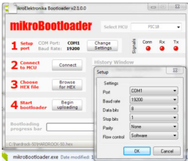
Change the Port to whatever COM port your HR50 registered as. Leave the rest of the settings alone and click OK. If you don't know which port your HR50 is on, start the bootloader with the HR50 powered off, note which ports are available. Shut down the bootloader, power up the HR50, restart the bootloader and the new port in the list will be the HR50's port.
