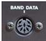
Yaesu FT-1000MP BAND DATA connector
