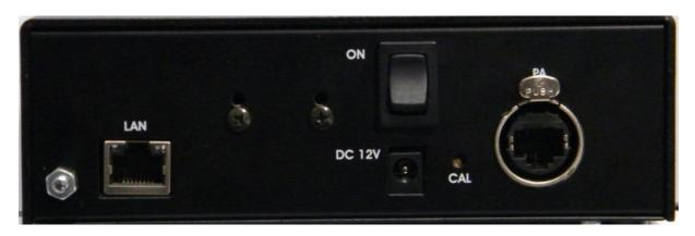
LAN - Standard RJ45 connector - LAN Interface for remote access
