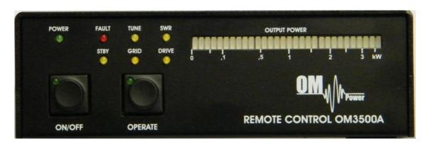
ON / OFF - Standard ON / OFF switch. On state is indicated by green LED on the switch
