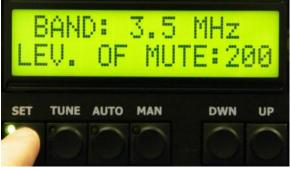
Then configure MUTE LEVEL for each band so it results in no power being transmitted by TX when performing TUNE procedure.
