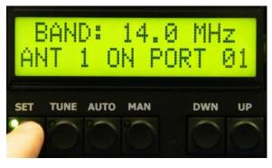
To finish Antenna switch configuration you can either press AUTO or MAN.
