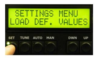
In the rare case of needing to restore factory default settings press SET and scroll using UP / DWN to LOAD DEF VALUES and confirm by SET.
