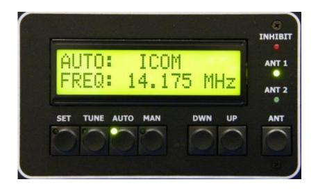
**INHIBIT** Indicates interruption of transmission during the tuning process of the PA.
