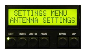
By pressing SET and scrolling to ANTENNA SETTINGS and confirming by SET you get current band and its antenna selection.
