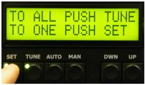
In the case of resetting a single parameter use UP / DWN to select which option and confirm by SET.
