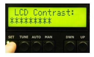
By pressing Up or DWN you can vary contrast of the LCD display. Finally press SET to confirm selected value.
