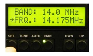
To enter Manual mode of the PA press MAN. By pressing MAN repeatedly you select BAND and band segment. You can control the segment or band by scrolling the UP / DWN buttons.
