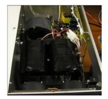
This is the final position of the transformer and the connector plug.
