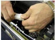
Plug the connector on the transformer into the one on the wiring harness. It is keyed so that it cannot be plugged in backwards. Make sure that the connector halves are pressed together until the lock tabs snap in place.
