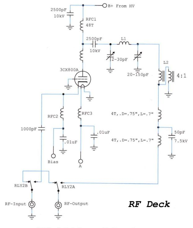
RFC3: 3-3-3 Turns, 61 Binocular Core RFC2: 5-5-5 Turns, 61 Binocular Core
