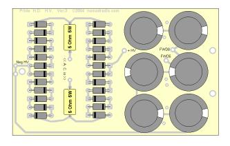
Now insert the other twelve rectifiers, the ones that point to the left. This is a good time to insert the two 5-ohm 5-Watt resistors, also.
