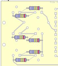
Next, bend the leads parallel on six of the 240k 2-Watt bleeder resistors.
