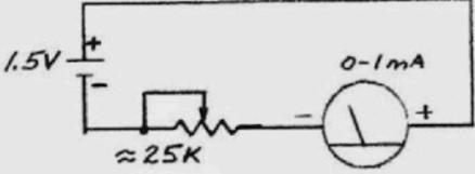
Hook up the meter as shown above. Adjust the potentiometer so that the meter reads 1mA. Remove the potentiometer from the circuit and measure its value with an ohmmeter. Use this value with the equation on the next page to determine R meter.
