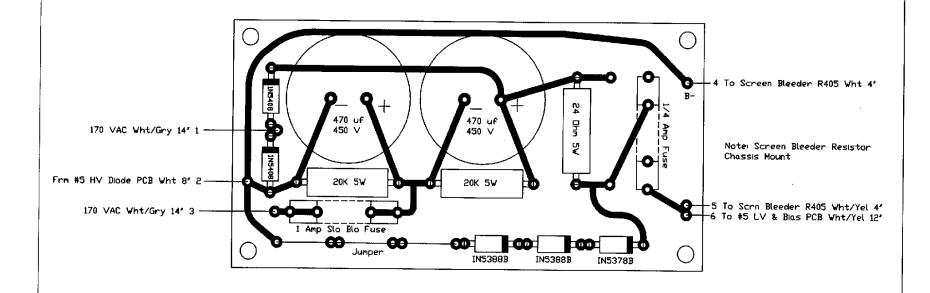
Note: All Trace Holes .0625 dia. Four Corner Holes .1875 dia QRD Technologies, Inc. Screen Supply PCB Model HF-2500DX/HF-3KDX Part No. 06130 Drawn by! Ray V. Connin March 17, 2000
