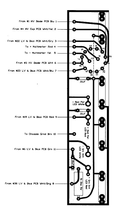
Note: All small holes .0625 dia. All large holes .1250 dia. QRD Technologies, Inc. Meter Switch PCB Part No. 06113 Model: HF-2500DX/HF-3KDX Ray W. Connin October 23, 1995 Rev. 2: 02/10/97
