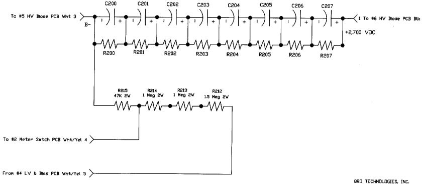
C200 - C207 470uf 450V R200 - R207 50K 5W QRO TECHNOLOGIES, INC. HV Capacitor PCB Model: HF-2500DX/HF-3KDX Part No. 06111 Drawn by: Ray W. Connin October 8, 1995 Rev. 1: 5/7/96
