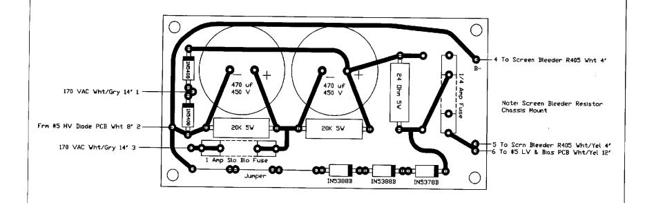
Note: All Trace Holes .0625 dia. Four Corner Holes .1875 dia GRU Technologies, Inc. Screen Supply PCB Model: HF-2500DX/HF-3KDX Part No. 06130 Drawn by: Ray V. Connin March 17, 2000
