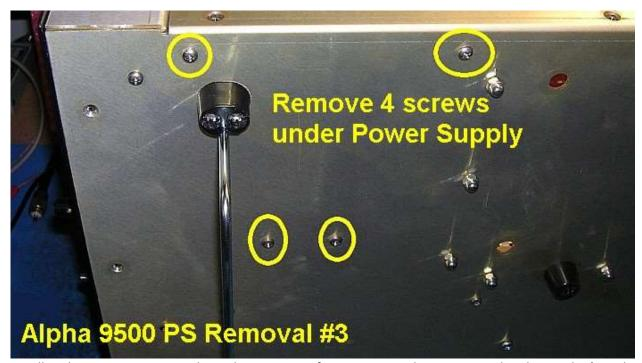
Install replacement power supply stack in reverse. If you mis-mate the gray 20 pin headers or don't push them all the way on, then the amplifier may not turn on.
