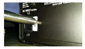
Pull out the panel to extract the voltage change system with the corresponding cables.
