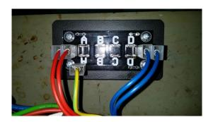
Connect cable "1" to one of the spade lugs labelled "A" Connect cable "2" to one of the spade lugs labelled "D"
