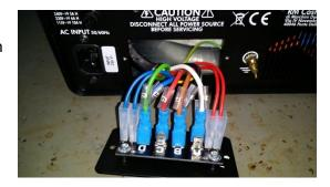
With pliers, remove all the numbered cables from the panel. Do not pull the cables to disconnect the connector.
