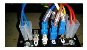
Connect cable "5" to one of the spade lugs labelled "C" Connect cable "6" to one of the spade lugs labelled "D"
