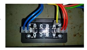
Connect cable "1" to one of the spade lugs labelled "A" Connect cable "2" to one of the spade lugs labelled "B"
