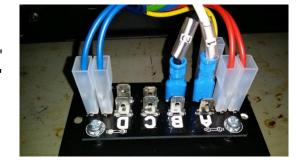
Connect cable "3" to one of the spade lugs labelled "B" Connect cable "4" to one of the spade lugs labelled "C"
