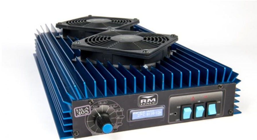
Figure 1: HLA-305V HF Amplifier, with cooling fans.
