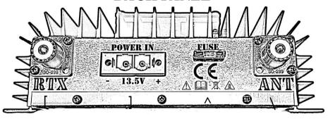
[  $TX/TX~50\Omega$  Connector to be connected to your radio transceive MAXIMUM POWER-IN 10W
