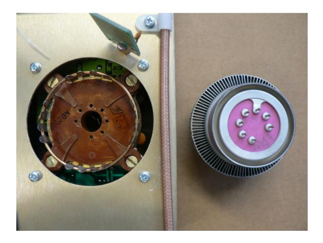
Before assembling the new tube it must be "conditioned".
