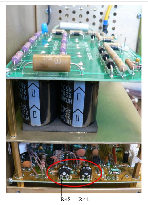
After assembling the new tube it would be necessary to adjust the plate current. Run the Alpin 100 without cover and connect to a transceiver.
