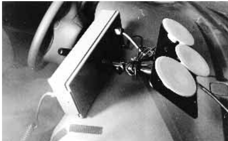
Figure 11— Seen from outside the GEO Metro, the suction cup mounting securely holds the PowerTalk remote head
