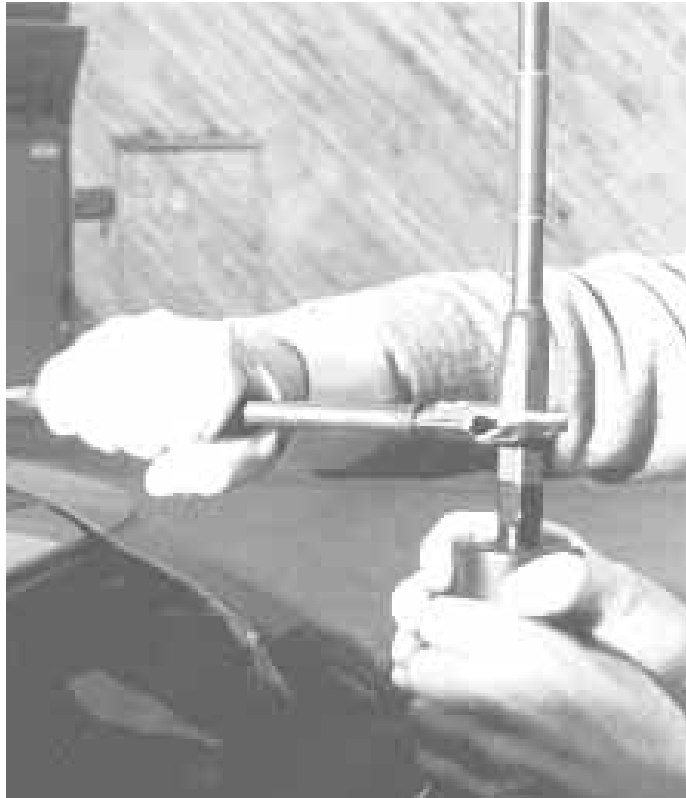
Figure 16 — One person grasps the rubber antenna base to prevent its turning while a second person tightens the whip with a wrench
