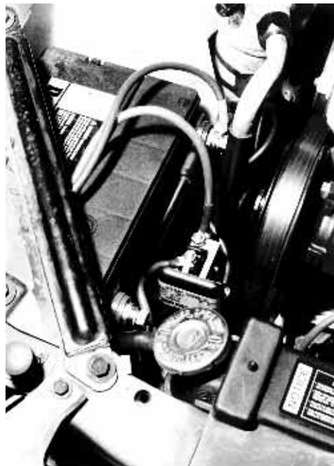
Figure 19 — The solenoid mounts next to the Cadillac battery
