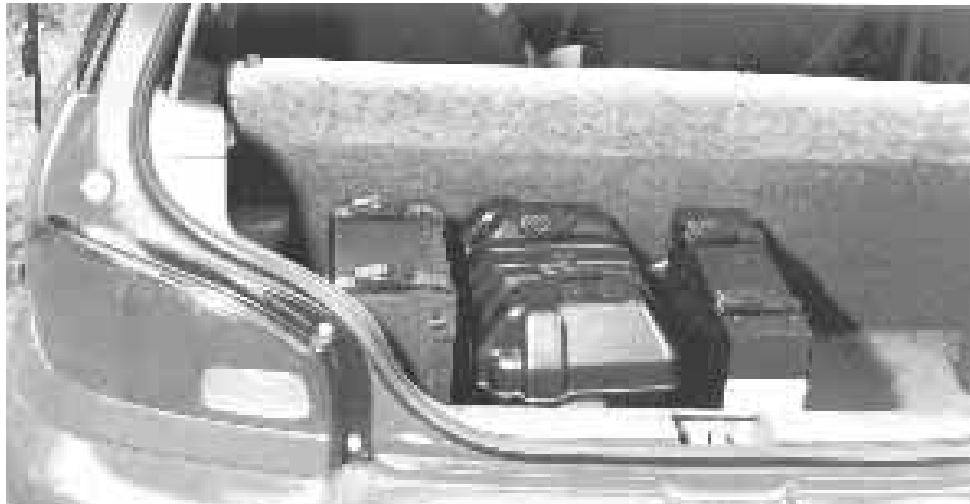
Figure 18 — The 500-watt system fits neatly in the rear compartment of the GEO Metro
