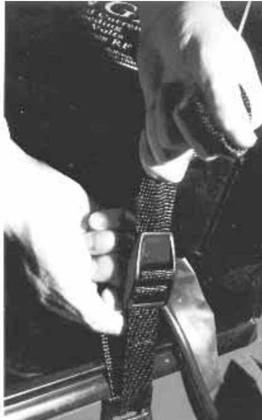
Figure 14 — Tighten straps to maintain pressure on suction cups. Plan to retighten straps after dri-
