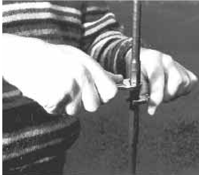
Figure 15 — Tighten the two sections of the whip with wrench- es
