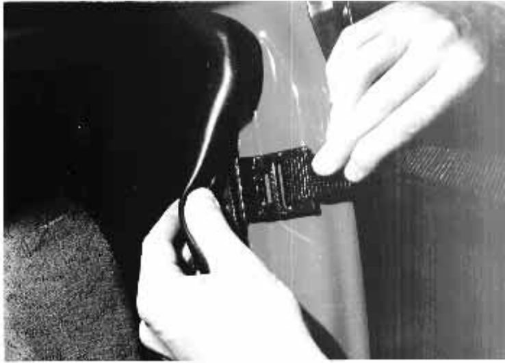
Figure 2 — Hooks can attach beneath door gaskets
