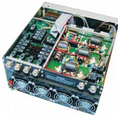
Photo 3: The six MOSFETs on the right are arranged as three push-pull pairs. On the left is the auto ATU section.
