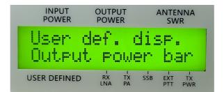
User Defined display item is assigned to output power bargraph. This bargraph has full scale of 350W.
