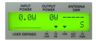
Amplifier can be activated by RF signal from transceiver or by remote PTT signal (if external PTT mode is active).
