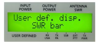
User Defined display has now been assigned to antenna SWR bargraph. This bargraph has full scale of SWR=3 and zero at SWR=1.
