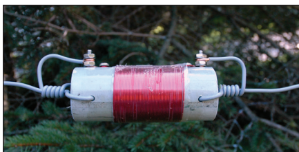
The DX-EE uses inductive loading on the 40/20 meter wires to reduce the overall length to just 40 feet.
