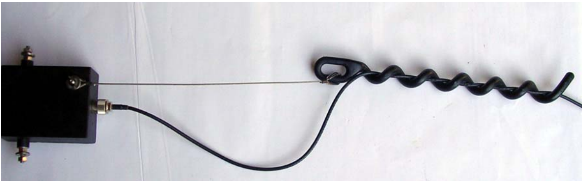
Balun with coax attached and wrapped around strain relief “corkscrew”
