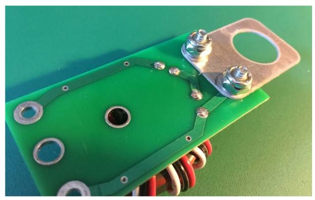
Bend the coax mounting bracket 90 degrees up as shown. Use a firm surface for a nice clean bend.
