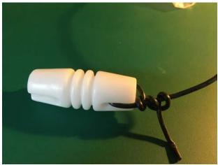
Crimp and solder antenna wire and tie the other end to the end insulator.
