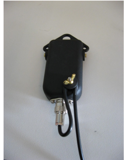
Above: Bushcomm Balun showing coaxial strain relief feature***
