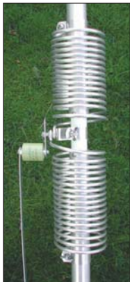
Left: Close-up of the 40m (top) and 80m loading coils.
