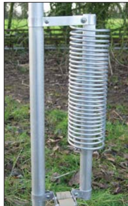
Left: Close-up of the 40m (top) and 80m loading coils.
