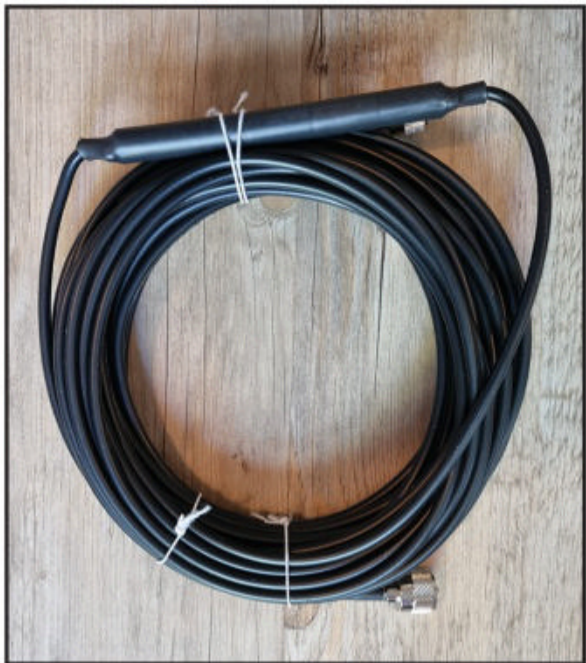
Photo H. The kit even includes a length of coax with a built-in RFI choke.
