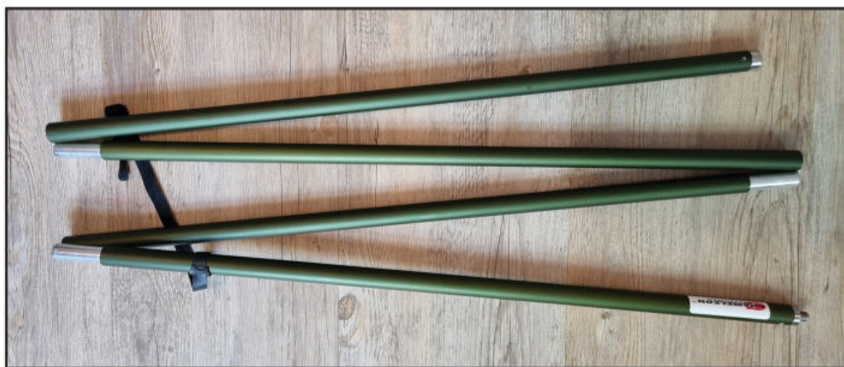
Photo F. The collapsible whip extension allows operation on 1.8-54 MHz with just an antenna tuner.
