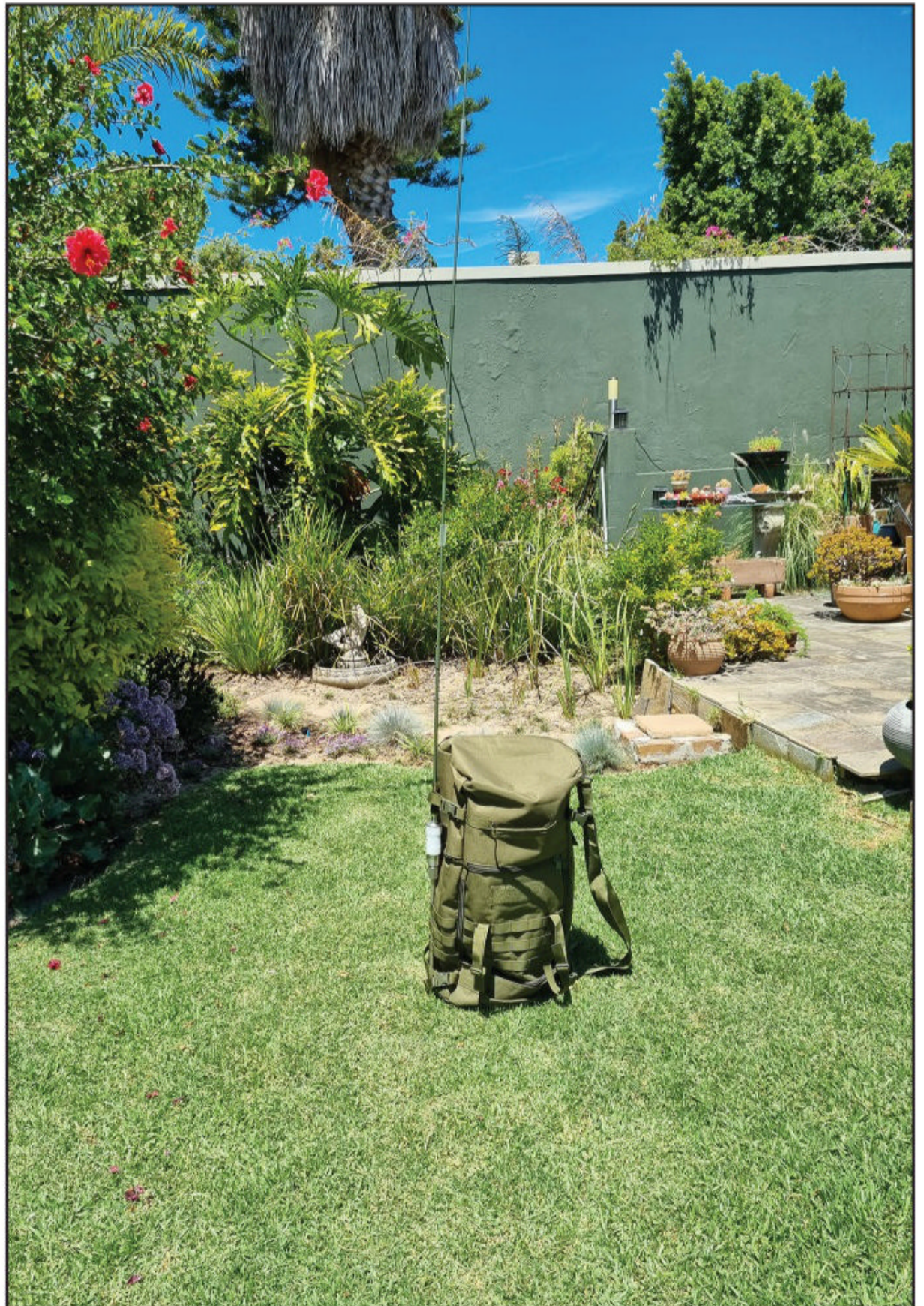
Photo I. The CHA MPAS 2.0 system set up in the manpack configuration.
