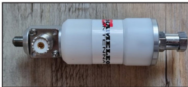
Photo C. The Hybrid-Micro impedance transformer is the heart of the Chameleon antenna system. The feedline and antenna elements attach to it and it serves as a base for several configurations.
