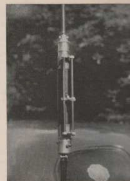
Fig. 15-17 — Close-up of the slider-tuned loading coil.
