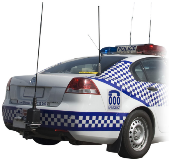
Figure 5: Rear-mount location on sedan vehicle
