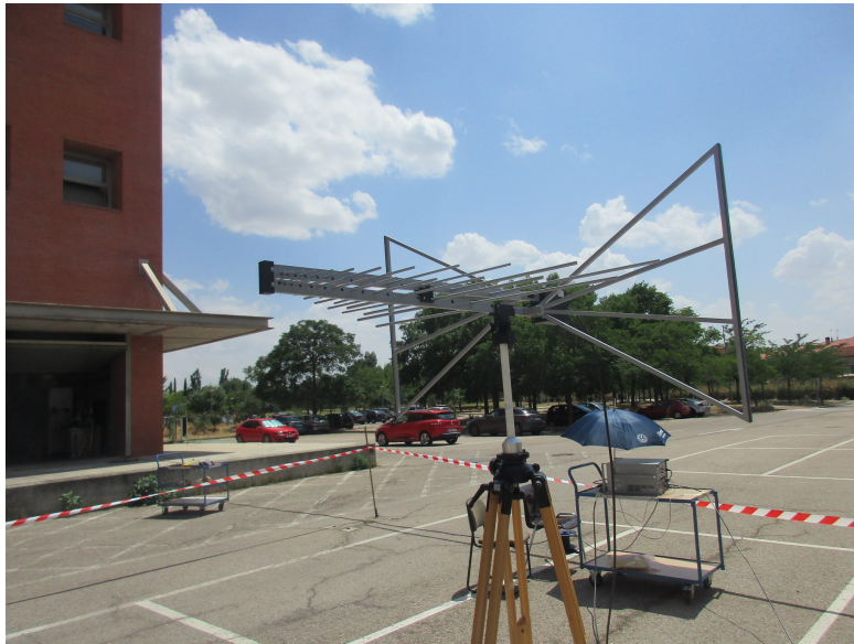
Figure 6: EMCO 3142 transmitting antenna
