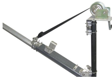
Four Bolts to be removed to allow for pivoting
