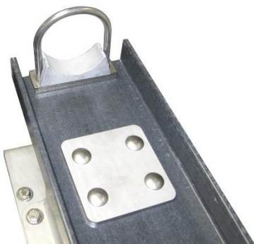
Top of Insulated Channel Showing U-Bolt installed The Thick Spacer is on the front side The Thin Spacer is on the rear side
