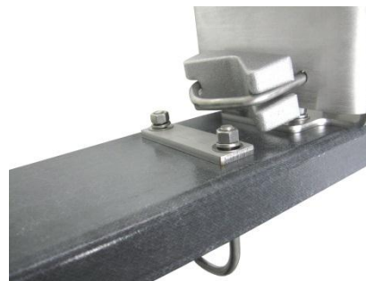
Rear and Front views showing the U-Bolt located at the Bottom of the Insulated Channel The Thick Spacer is on the front side, the Thin Spacer is on the rear side
