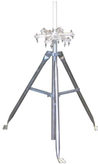
Figure 1 - Using a temporary tripod and mast for assembly at ground level
