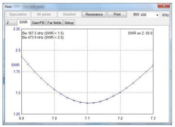
According to the books, dipoles and verticals resonate on every odd harmonic. This means that according to the maths, our element tuned for 7.1 MHz should also be resonant on 21.3 MHz. If it were that simple, I wouldn't be writing this.
