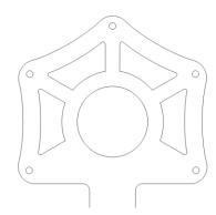
Ground Plate: This is made from 3mm aluminium with a single bend for the SO239 assembly and 5-holes for ground radials. I personally tap these
