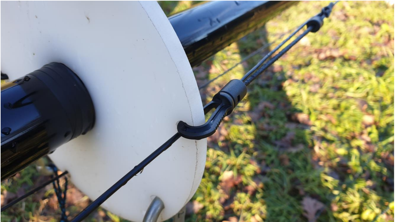
Showing the 80m element coming through the 3 rd guy point and continuing to left of picture with carabiner holding tension on the plate.
