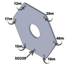
For every band (not 40m) create a 6cm loop and secure with electrical tape (don't add 6cm to the cut, just create it after cutting)
