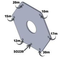
Although it does not matter which element you start with, let us start with the 20m element for sake of argument. Connect the fork-connector to the aluminium driven plate by slipping a washer over the top of your fork connector and secure with a supplied wing nut.
